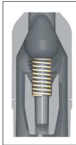
Figure 7: Backpressure valve (courtesy of Weatherford)
