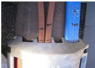
Figure 13: Control lines externally clamped to the tubing.
