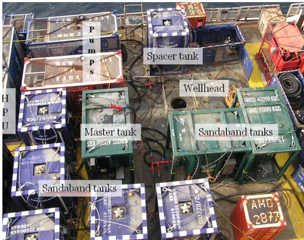
Figure 11: Sandaband® Rig-up. Source: Embla Post-job presentation by Conoco Phillips
