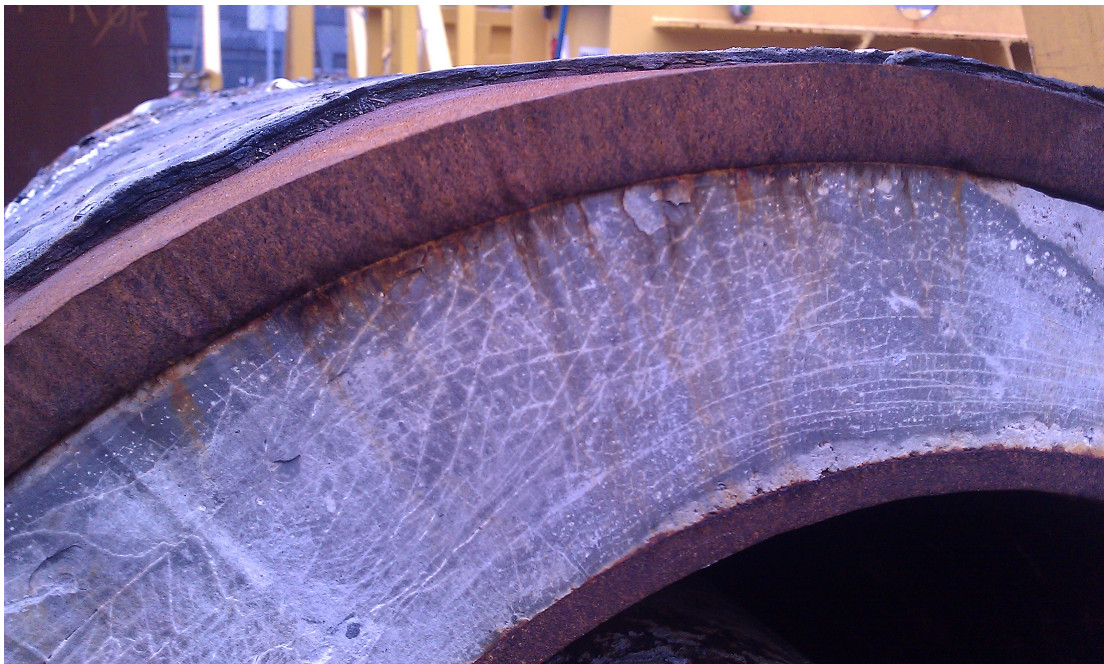
Figure 7: Cut of casing and cement with abrasive water jet technology.
