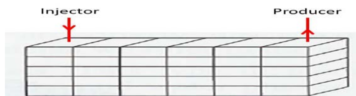
Figure 4.2 Schematic representation of the synthetic model and the wells (not to scale).
