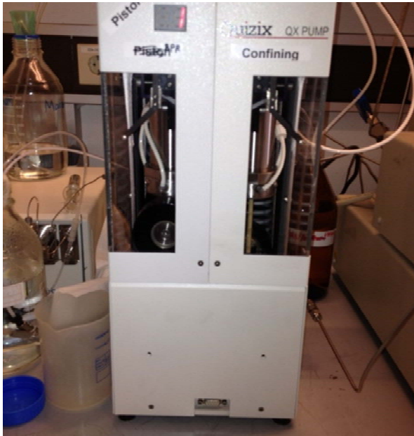
Figure 6.2: High pressure Quizix QX pumps controlling the piston (axial) pressure and confining pressure.
