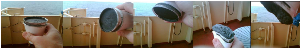
Figure 22: Sandaband in solid phase refloated to liquid phase. [Sandaband presentation from P&A forum 09.06.2011]
