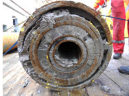
Figure 19: Multistring conductor cut performed with abrasive water technology. [www.nca.com]
