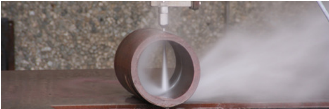
Figure 20: Abrasive water cutting through steel. [www.nca.com]
