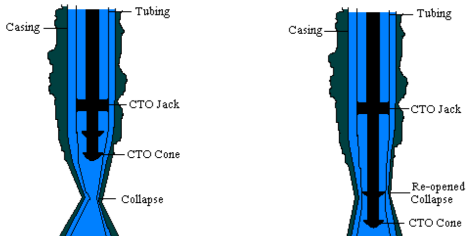
Figure 35: Re-opening collapse with Casing/Tubing Opening tool.
