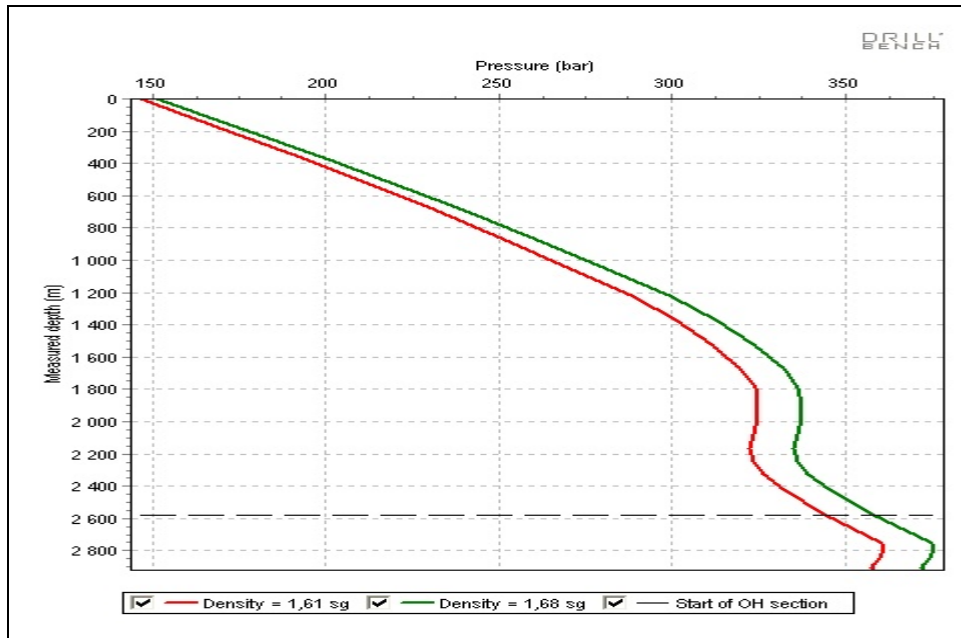
Figure-A.1: Pressure in drillstring for two mud weights.
