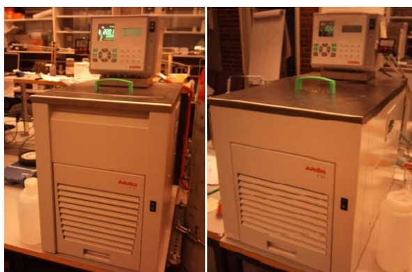
- Figure 3.2.1: The cooling baths. Model: Julabo F33 (Left) and Julabo F34 (right)
