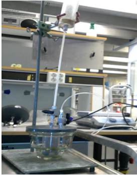
Fig 3.6. Saturation of core under vacuum pressure
