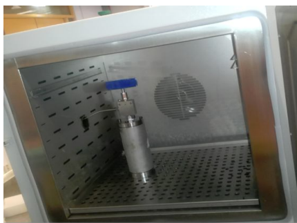
Fig 3.12. Aging core under reservoir temperature condition (130 0 C)
