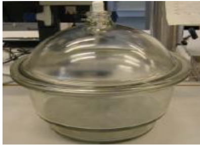
Fig 3.10. Establishment of initial water saturation using desiccator
