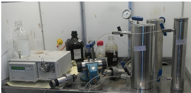
Fig 3.5. Toluene + Methanol cleaning core set up
