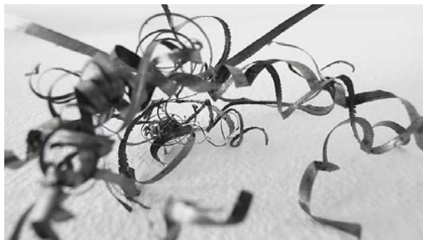
Figure 2.6: Metal debris, also known as swarf (Borrowed from zimoun.net)
