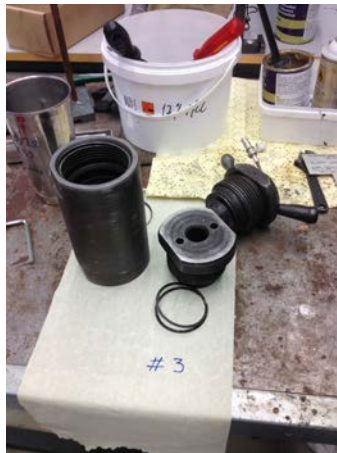
Figure 5.1: Container that is used in the Ultrasonic Cement Analyzer
