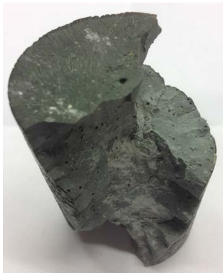
Figure 5.16: Sample no. 107 after UCS test
