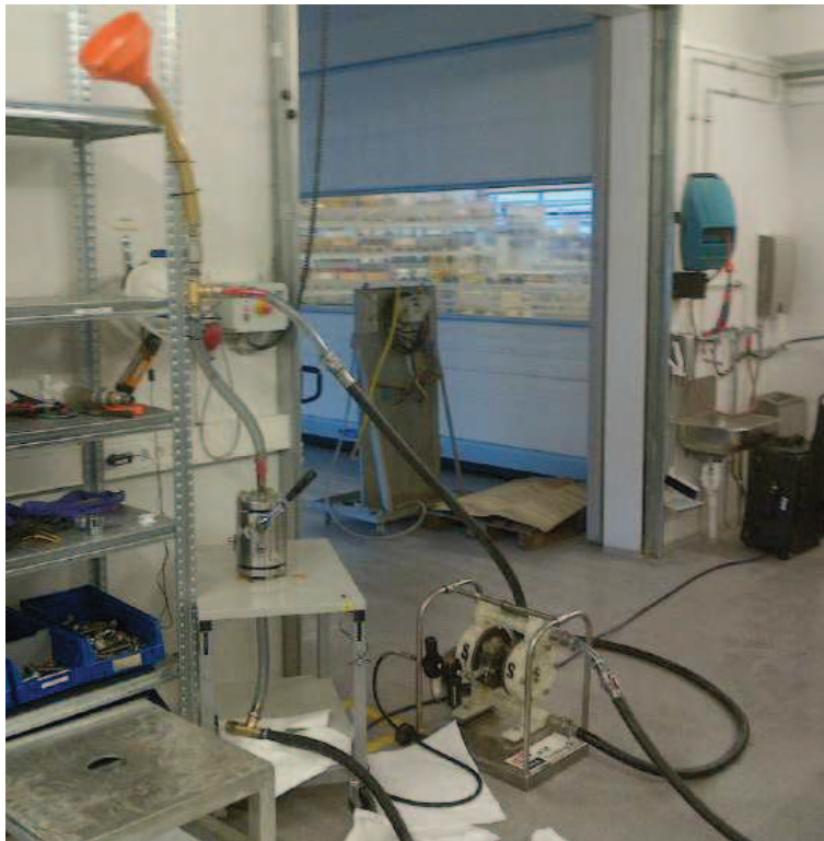
Figure 17 - Picture of the mini flow loop before filled with diesel.
