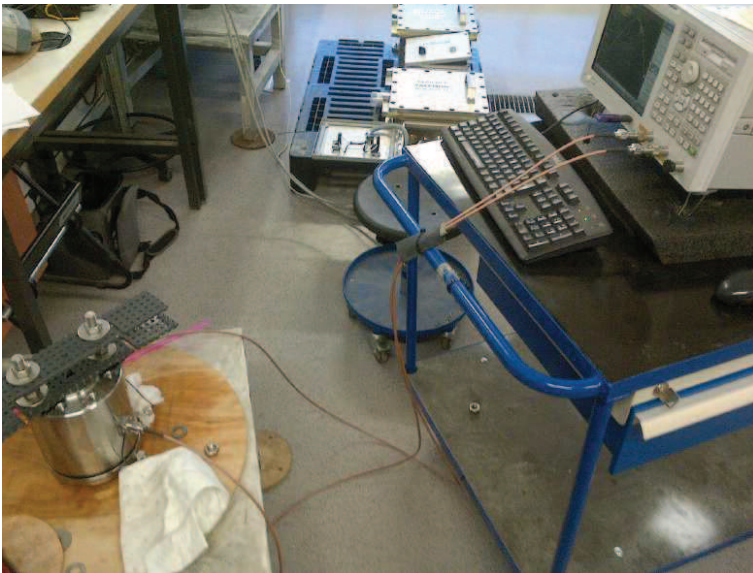
Figure 16 - The used network analyzer connected to CFRS sensor used in measuring the resonance frequency.
