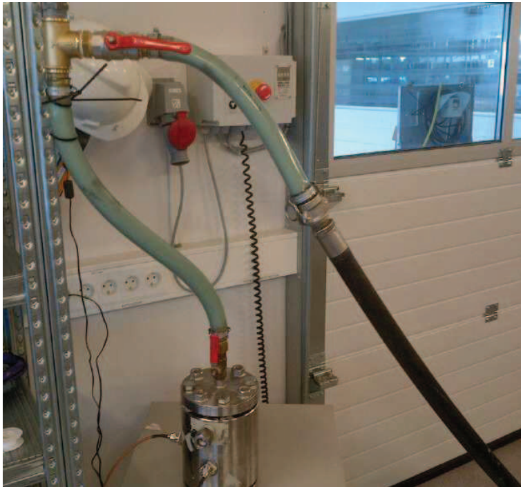
Figure 15 - Picture of the mini flow loop while circulating diesel and air.
