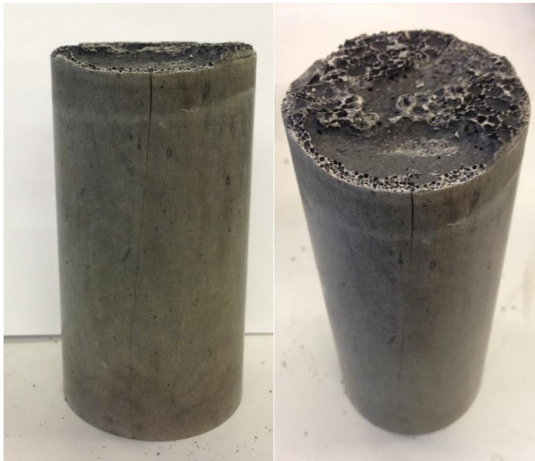
Figure 6.10: Sample no. 115 D showing a clear crack throughout the sample
