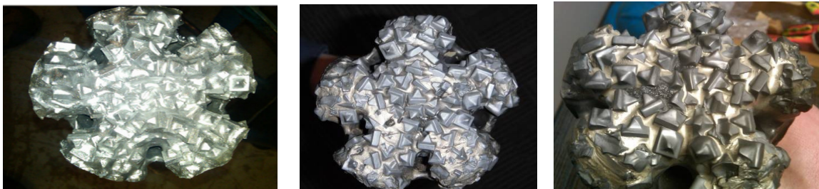
Figure 36: Wear down of cutter with Glyphaloy inserts [76].
