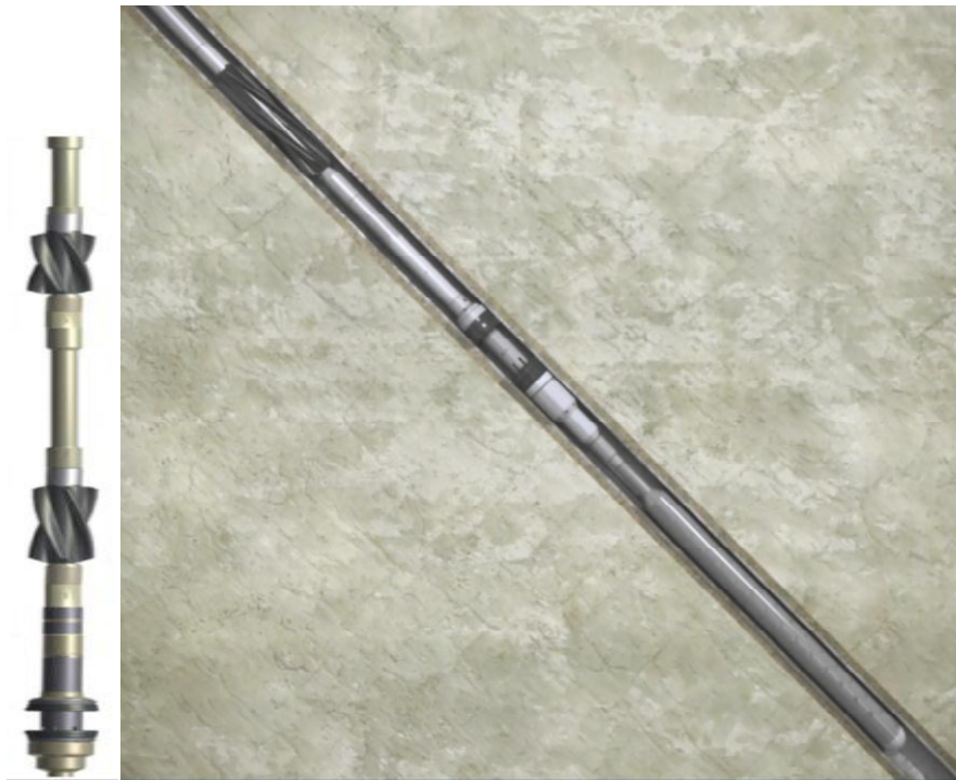
Figure 38: HydraWash [13]. To the right one see the top of the BHA, while the bottom is located on the left picture.
