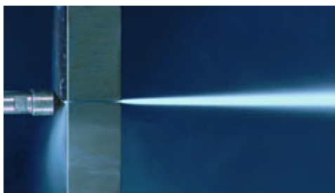
Fig 15: [34] Abrasive water jet cutting through steel
