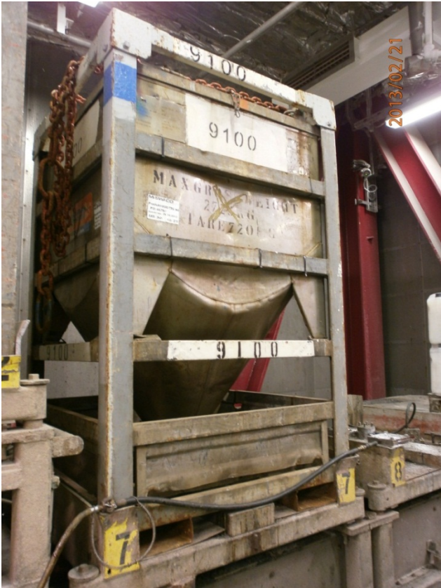
Detail of tank with chains for crane lifting
