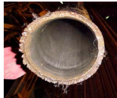
Figure 91 Cut performed with JRC Jet Cutter [15]
