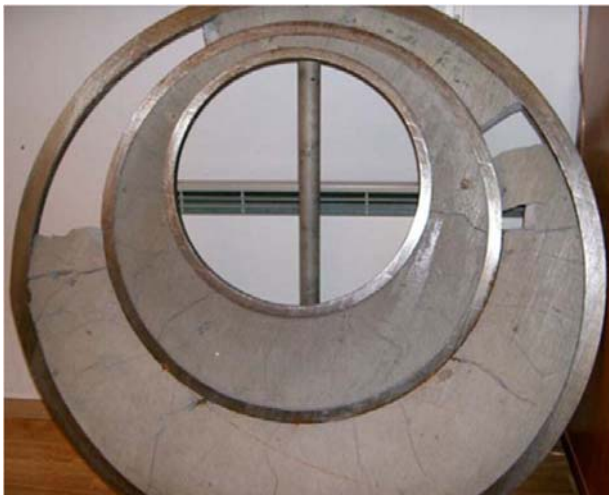
Figure 56 Cracks in the cement [33]
