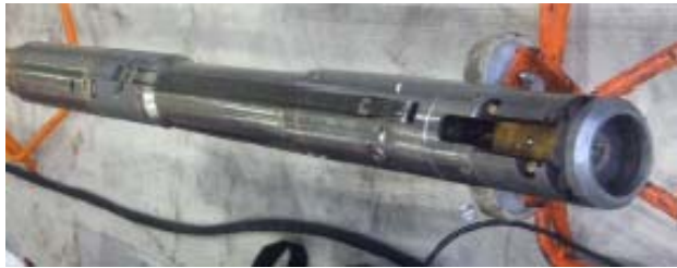
Figure 19 Picture of 7 inch downhole electric cutting tool [76]
