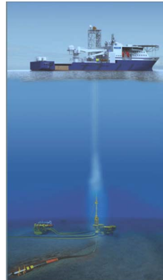
Figure 7 The RLWI vessel is position above the well [27]
