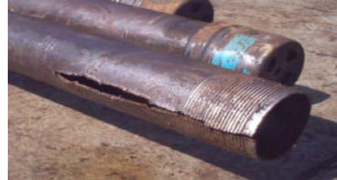
Figure 93 Tubing recovered with splitshot [15]
