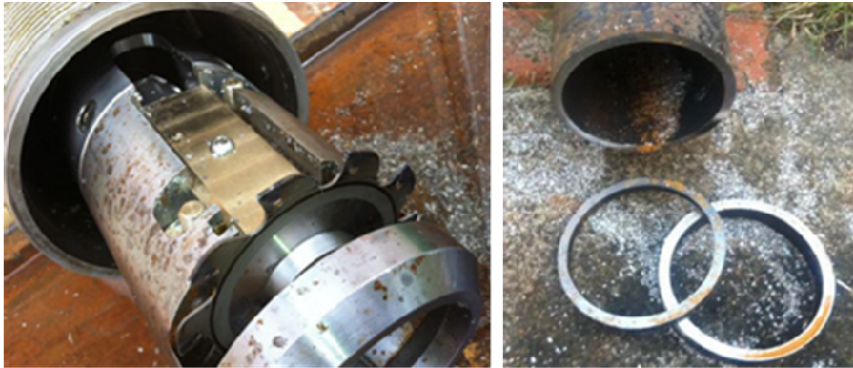
Figure 99 Picture and cut performed by 7” DECT [76]
