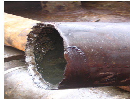
Figure 94 Cut performed with Plasma Cutter [49]
