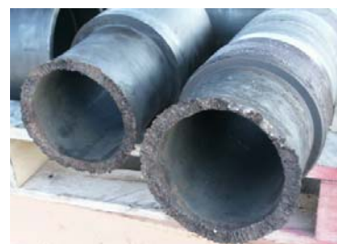
Figure 92 Cut performed with Power Cutter [49]
