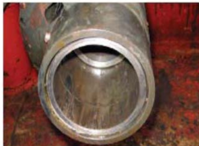
Figure 96 DECT tool anchoring system and ESP Packer Mandrel after cut [1]
