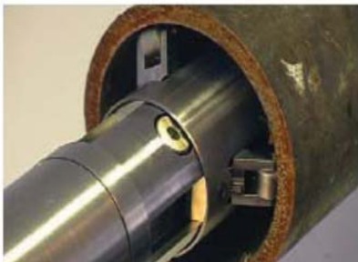
Figure 96 DECT tool anchoring system and ESP Packer Mandrel after cut [1]
