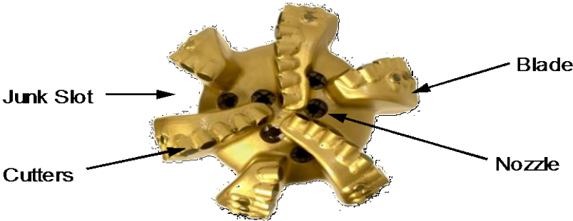
Figure 2.3: PDC bit with cutters and treated with oxy acetylene[2]
