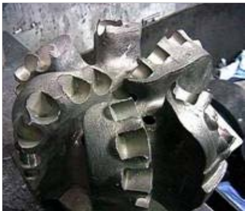
Figure 2.1: PDC bit without cutters inserted[2].
