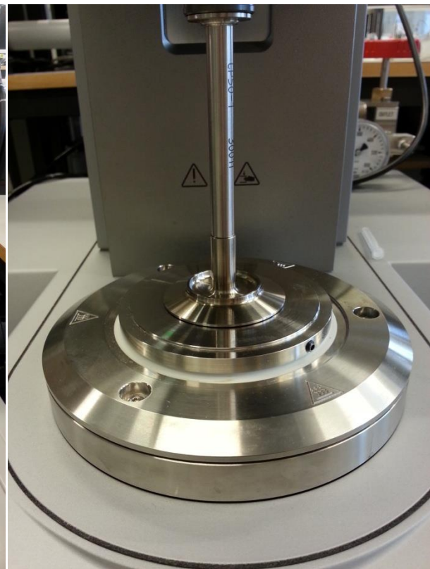
Figure 14: A close-up picture of the Plate-and-Cone (CP-50-1) configuration at measuring position.
