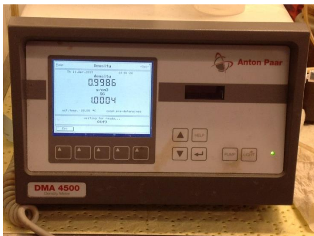
Figure 12: Picture of the Density meter as it is measuring the 1g/l CMC. Photographed by Kim Flatrårker.
