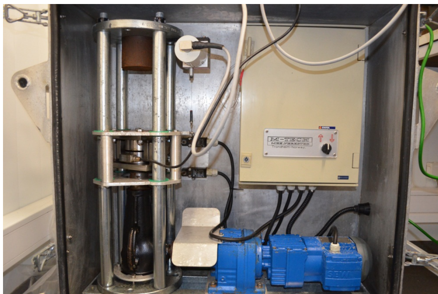
Figure 35. “Kompis” – pressure machine for field studies.
