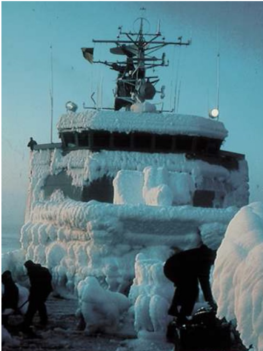
Figure 19 Icing on K/V Nordkapp 1987 (Løset et al. 2006)
