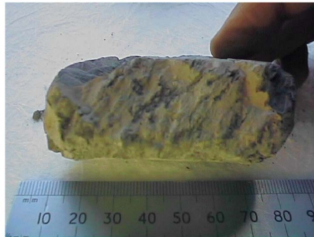
Figure 32: Tabular cavings (Bradford et al., 2000)
