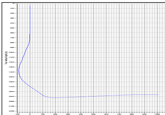
Figure 5-2: Section view of well A-11 [25].
