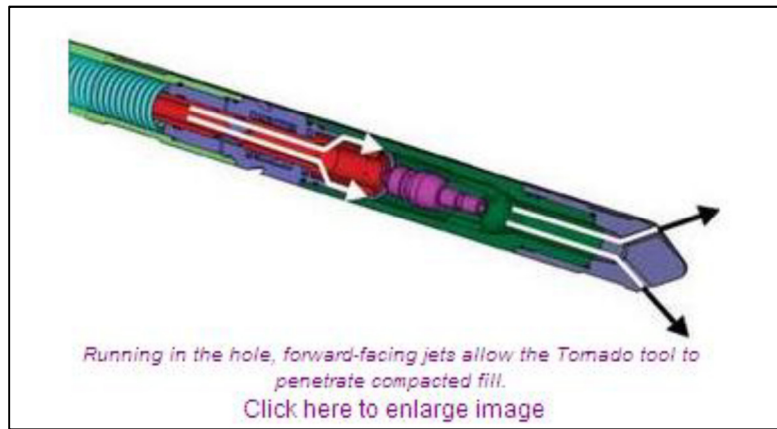
Figure 2-1: Sand / Fill clean out - Tornado tool [16]
