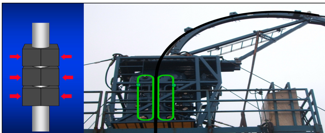
Figure 1-5: CT Injector Head and Gooseneck [8].
