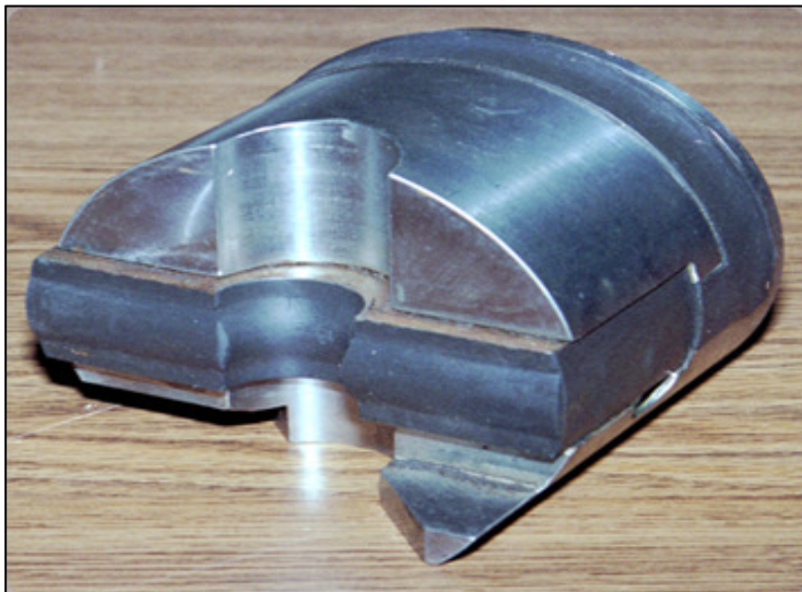
Figure 1-14: CT BOP's Pipe ram assembly [8].
