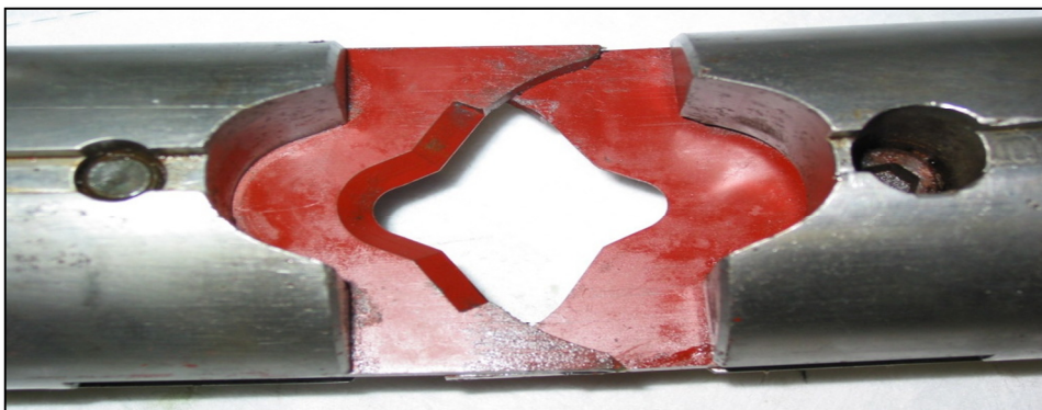
Figure 1-12: CT BOP's shear rams [8].
