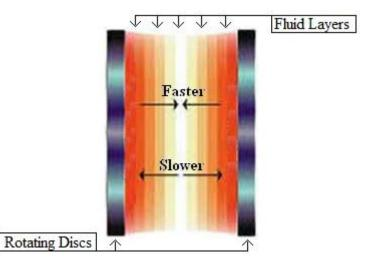
Figure 36 Successive layers of fluid between the two rotating discs. Figure taken from [31].
