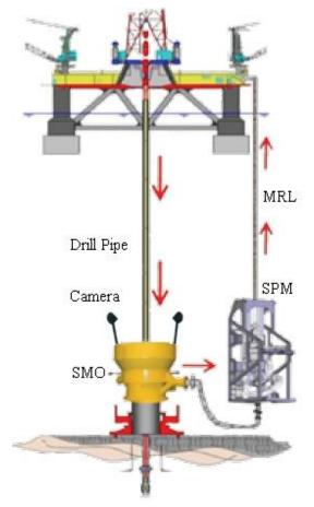
Figur 8 RMR<sup>®</sup> Setup. Figure is taken from AGR.
