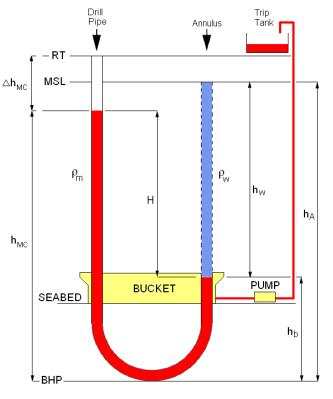
Figure 31 Illustration of the U-tube effect
