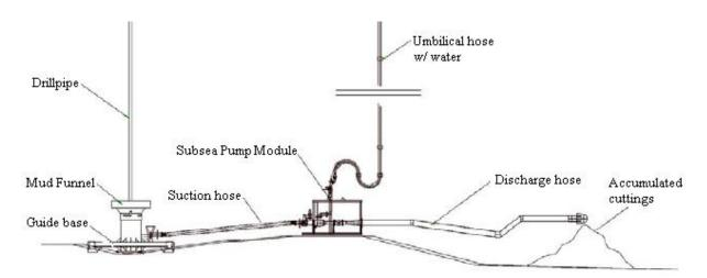
Figure 4 Cuttings Transport System schematic for IKMs injector technology. Figure is taken from IKM.
