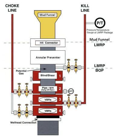
Figure 22 The subsea arrangement of an 18 <sup>3</sup>/<sub>4</sub>" BOP stack with four rams, LMRP and Mud Funnel. Figure is taken from reference [25] and modified.
