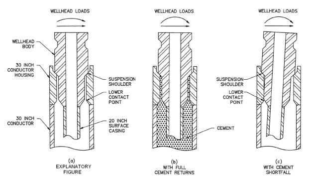
Figure 9 Effect of cement shortfall around wellhead. Figure is taken from [18].
