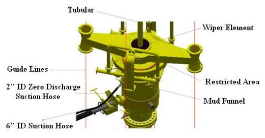
Figure 13 Zero Discharge Arrangement on top of Mud Funnel. Figure is taken from ORS.
