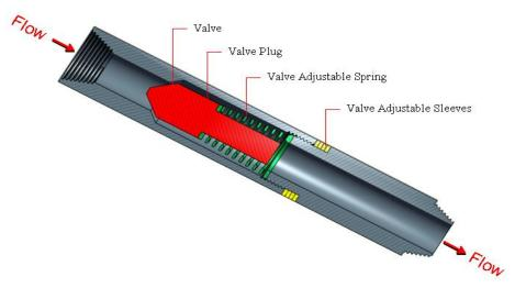
Figure 32 Schematic drawing of a Flow Stop Sub. Figure is taken from Baker Hughes [28].
