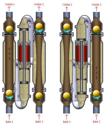
Figure 50 PG-MAPS hose diaphragm pump configuration for one double-acting actuator. Figure is taken from [34].
