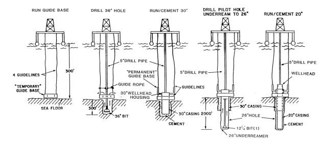
Figure 3 Schematic illustration of top hole drilling. Figure is taken from [9].
