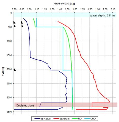
Figure 53 Drilling window for GFS showing a proposed drilling program for CRD and RD.
