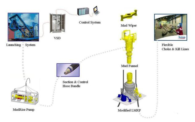
Figure 11 ORS Riserless Drilling System Components. Figure is taken from ORS.
