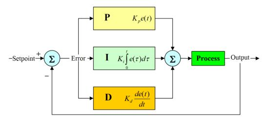
Figure 29 Block diagram of a PID-controller. Figure is taken from [27].
