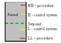
Figure 27 Level Control System alarm boundaries. Figure is taken from ORS.
