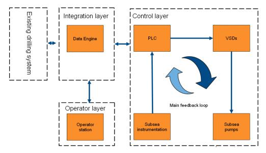
Figure 26 Action sequence architecture for the Control System. Figure is taken from ORS.
