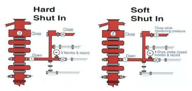
Figure 39 Shut-in procedures of BOP and rig manifold. Figure taken from WCS [40]
