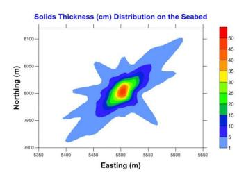
Figure 6 Deposition and accumulation of solids on seabed. Source: fluid-dynamix.com
