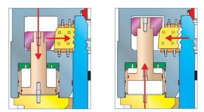
Figure 17 Magnified preview of the hydraulic control chamber for dog ring operation Left picture is locked position, whilst right picture is released position. Figure is taken from VetcoGray [22].
