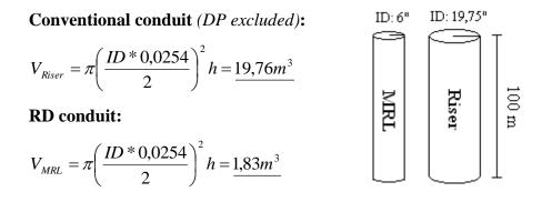
This is a significant difference with a total of 92.6 % saved conduit volume in favour of riserless. For large water depths this volume would be a comprehensive challenge in terms of the readily available fluid required for proper well control. Although well volume below mudline consists of approximately  $200 - 1000 \text{ m}^3$ , dependent on dimensions and depth, the conduit volume savings are highly noticeable in total volume requirements for large water depths.
