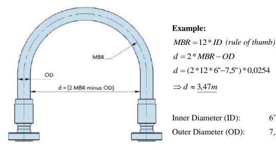
Figure 30 Required minimum distance before being affected of flexure. Figure is taken from [3].
