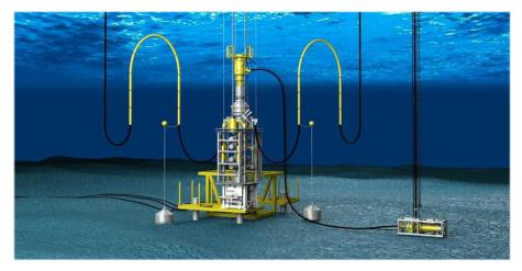
Figure 10 ORS Riserless Drilling arrangement Figure is taken from ORS.
