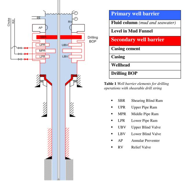
Figure 38 Well barrier schematic illustration of drilling with shearable drill string. Figure taken from [2]
