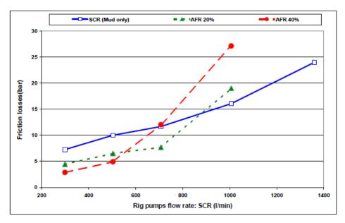
Figure 40 Dynamic friction losses inside the choke line. Figure taken from [41]
