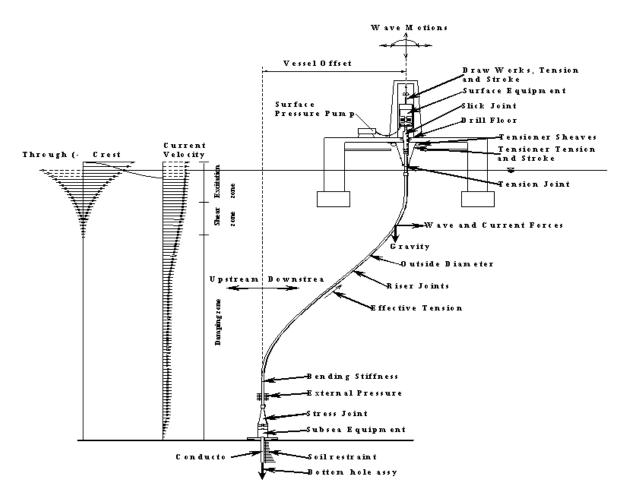
Figure 47 Riser geometry for a semisubmersible platform showing the acting forces. Figure is taken from [1].
