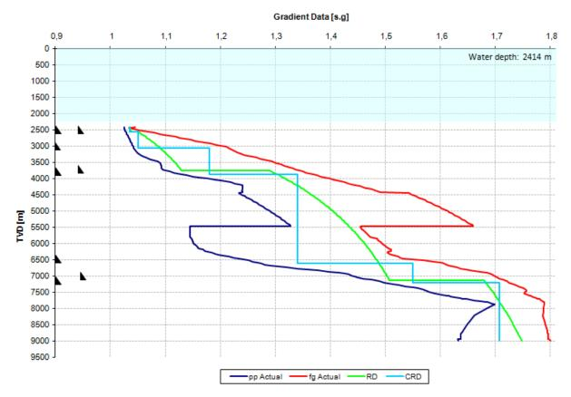
Figure 55 Ultra deep water and the advantageous use of a dual gradient approach.
