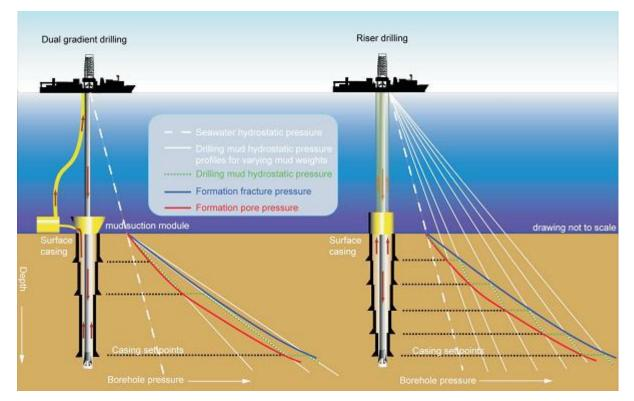
Figure 1 Principal drawing of the progression of pressure gradients along the well. Figure is taken from [5].
