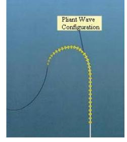
**Figure 21** *Pliant Wave Configuration of k/c hoses achieved by buoyancy elements. Figure is taken from ORS.*
