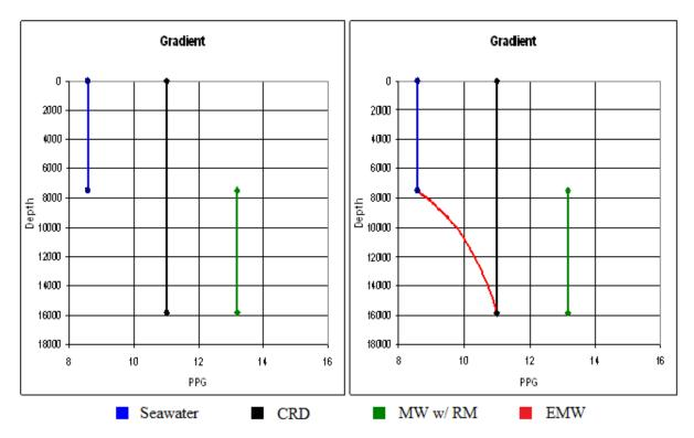
Figure 52 Illustration of the Effective Mud Weight (EMW) while descending. Figure taken from [65].
