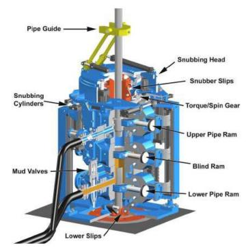
Figure 33 Schematic of a Continuous Circulation System unit. Figure is taken from Statoil's archive.
