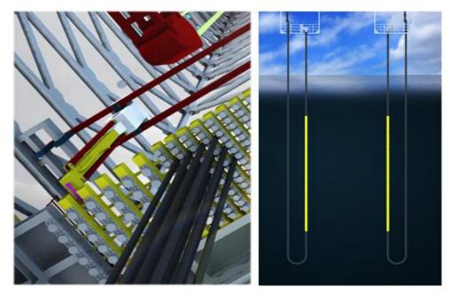
**Figure 24** The picture to the right shows the pre-built k/c hoses hanging from ORSs proposed basement deck. The picture to the left shows the k/c hose "stands" hanging from the finger table. Figure is taken from ORS.
