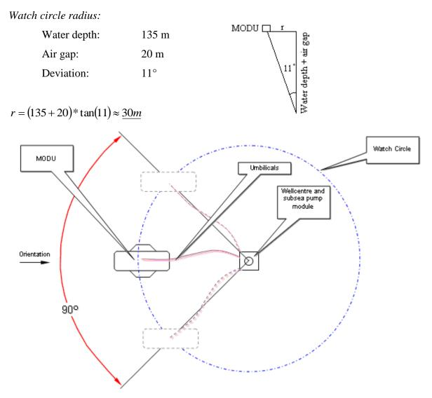
Figure 42 MODU watch circle for RD. The circle shows deviation allowance from well centre. Figure is taken from [42].
