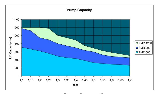
**Figure 37** *Pump efficiency graph for RMR*<sup>®</sup>600, *RMR*<sup>®</sup>900 and *RMR*<sup>®</sup>1200. For presentation purpose only. Data is taken from AGR.
