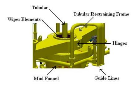
Figure 12 The Universal Wiper Element located on top of the Mud Funnel. Figure is taken from ORS.
