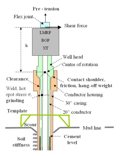
Figure 44 Subsea installation configuration for a typical subsea well. Figure is taken from [1].
