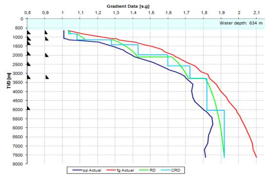
Figure 54 Clearly showing the effect of dual gradient in terms of compatibility within the drilling window.
