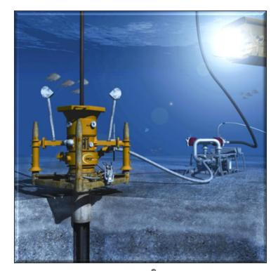
Figure 7 Subsea arrangement of the RMR<sup>®</sup> system. Figure is taken from AGR.
