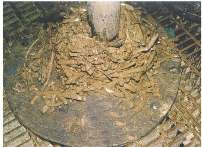
Figure 35 Ribbon shaped cuttings (source: Graham Mensa-Wilmot[13])
