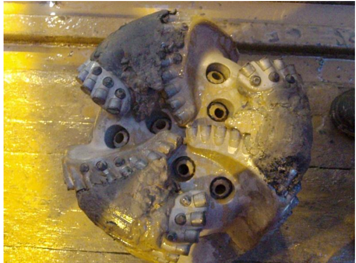
Figure 43 The FXG65R with 3 balled up waterways (Source: EOW report Zidane[3])
