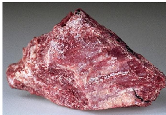
Figure 22 Smectite rock with absorbed calcium cation (Source: http://homepage.ufp.pt/biblioteca/ )
