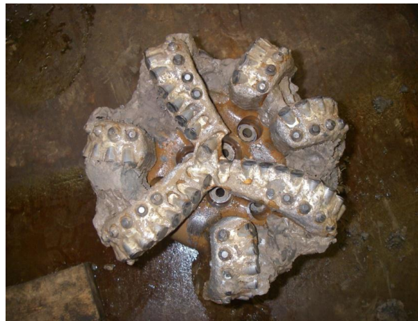
Figure 17 Partially balled up PDC bit (Source: Halliburton DBS)
