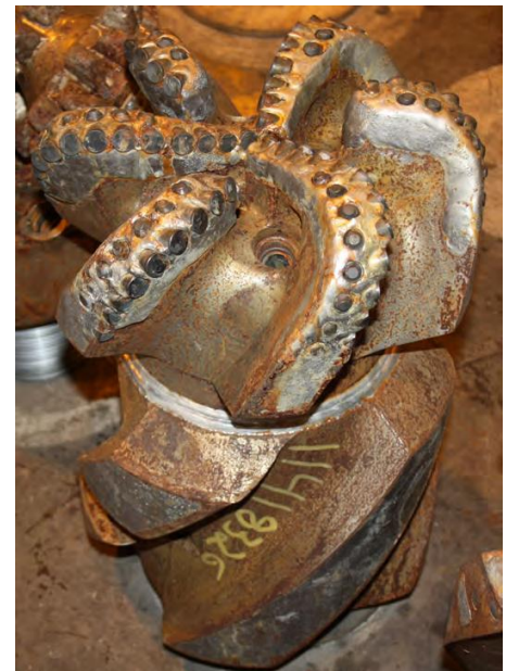
Figure 44 The FSFX653ZR anti balling bit (Source: EOW report Zidane[3])
