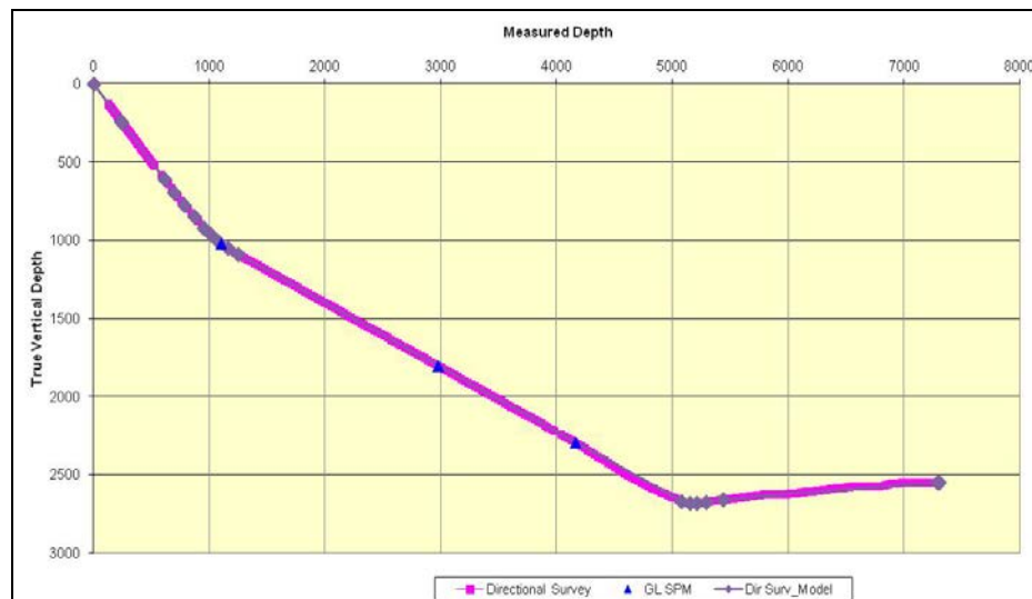
Figure 18 S-02 well directional survey filtering
