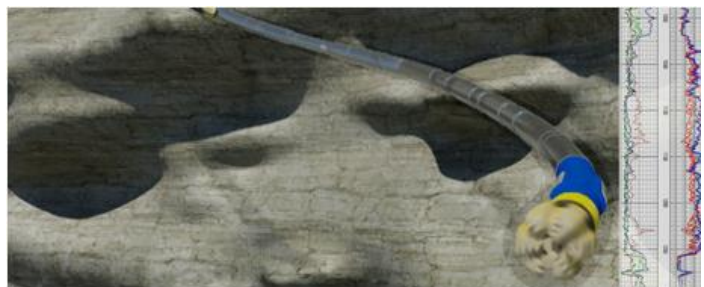
Figure 10.13: Steerable Drilling Liner System (Baker Hughes, 2012)
