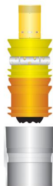
Figure 6.17: Indicator collar (bottom) with constriction in the middle. Plug at top (Weatherford, 2012)
