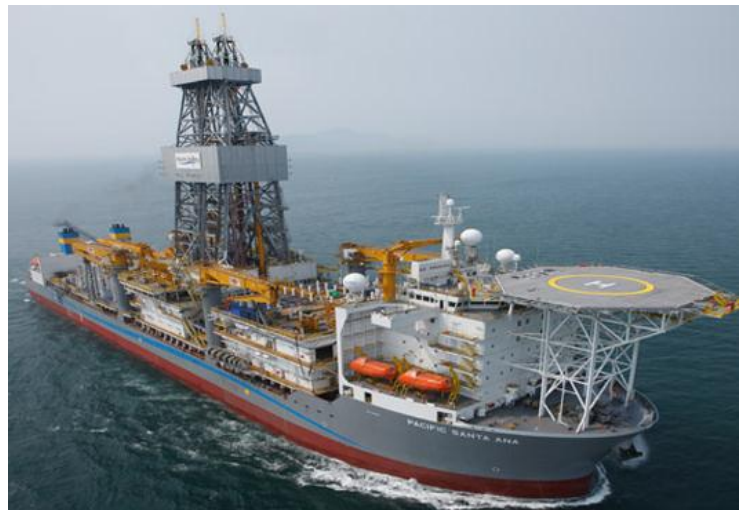
Figure 10.2: First drillship with dual gradient capacity, Pacific Santa Ana. Drillship built specifically for dual gradient operations according to Chevron specifications
