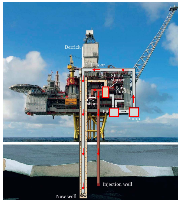
Figure 3.12: The circulation system for a drilling rig consists of pumps, drill string, drill bit, solids removal equipment, various pits and mixing system. Courtesy: V. Peikli, L.Ims, J.Ø.Ulriksen.
