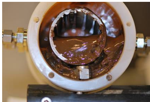
Figure 1.8: Picture taken from the front of a horizontal placed inner production screen covered with settled barite (brown-colored mass). The settling can cause plugging of the screen and hinder production. With this set-up, production can be simulated through the horizontally placed valves shown on the left and right side of the picture. Courtesy: G. Svanes.
