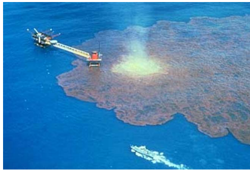
Figure 1.3: Stratification of the weighting material (sag) in the wellbore causing a dramatic blowout. Source: Maritime-connector.com
