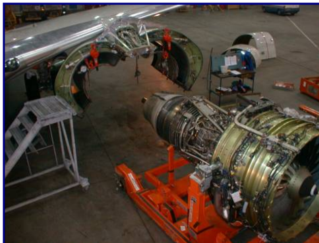
Figur 1 En CFM-56 motor klar for vedlikehold hos Pratt & Whitney, Norway Engine Center.
