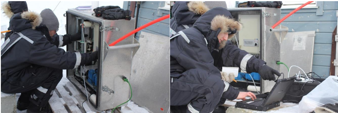
Figure 6 – Testing the ice cores in the portable compression rig “KOMPIS” (left) and recording the data (right) 15
