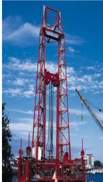
Figure 9 Traditional drawwork and a Ram rig system
