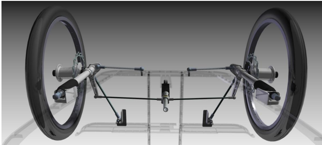
Figure 5- Front suspension on a 'tadpole' velomobile seen from above CAD model is based on Alligt Alleweder A4
