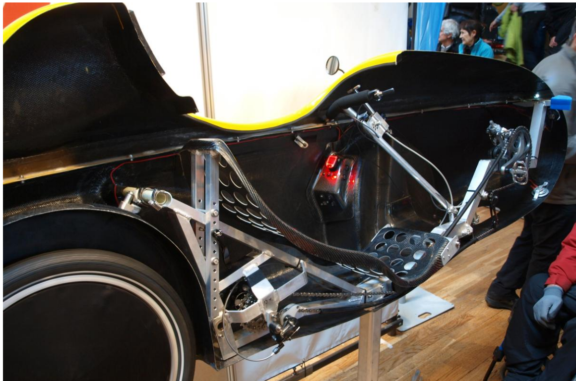
Picture 13 - A fast tadpole velomobile cut in half. Adjusting seat, steering and pedals takes a long time
