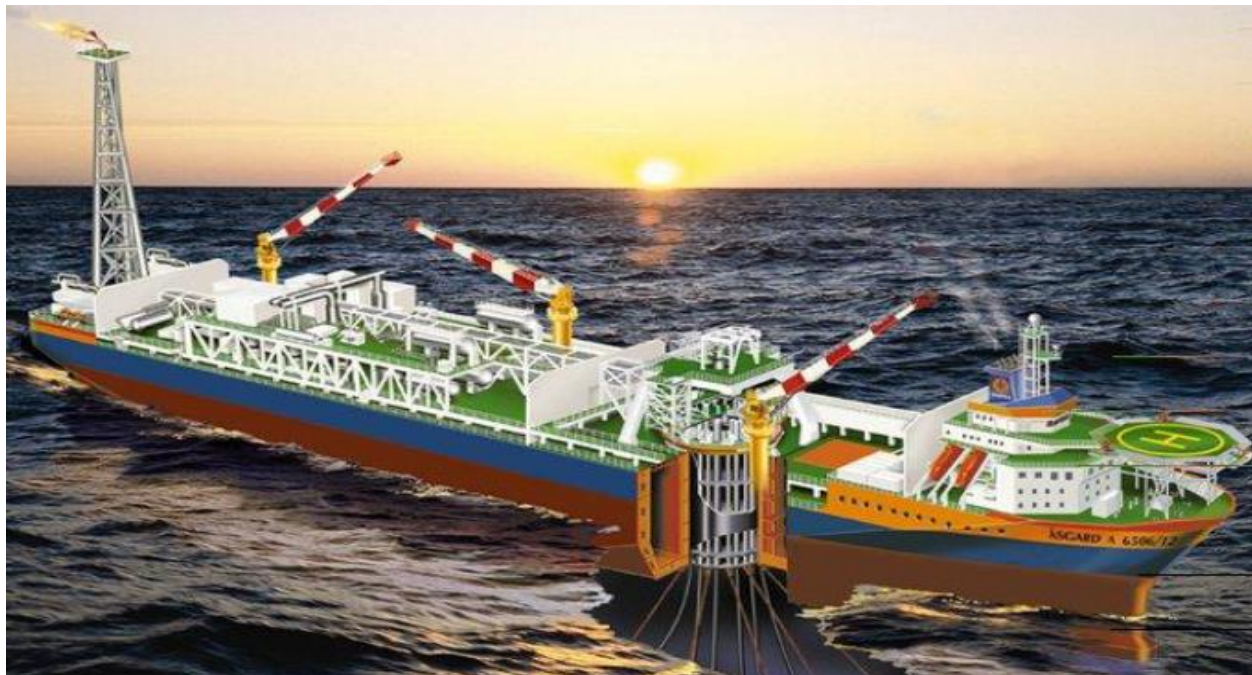
Figure 2.3 ÅSGARD A – Internal turret moored FPSO (Odland, 2012a)
