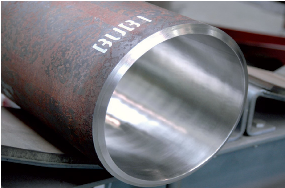
Figure 6.4 – Mechanically Lined BuBi® Pipe [BUTTING Catalogue, 2008]
