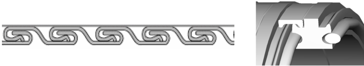
Figure 5.11 - Structure of Conventional Carcass and K-Profile Carcass [Nielsen et al, 2011]
