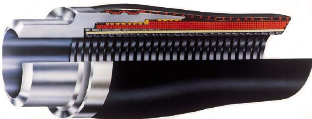
Figure 5.8 - Cross-section of Coupling Used with Bonded Flexible Riser [Antal et al, 2003]
