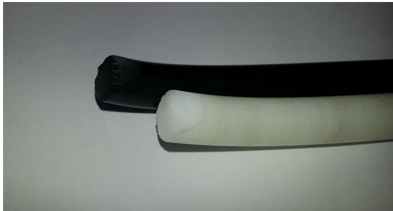
Pic 6-14: POM-C bending fracture
