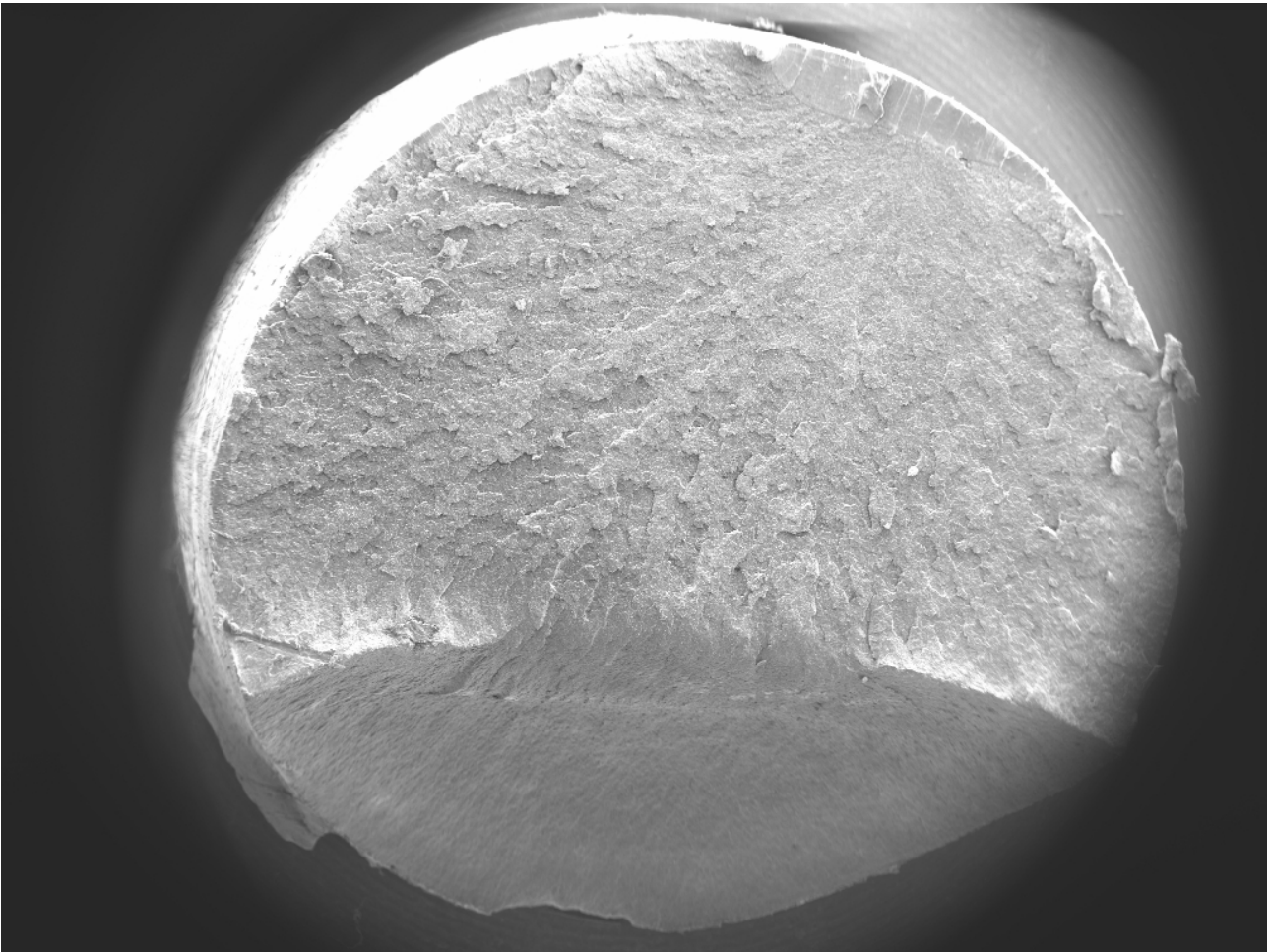
Appendix A5 (Bending experiment, fracture surface POM-C):
