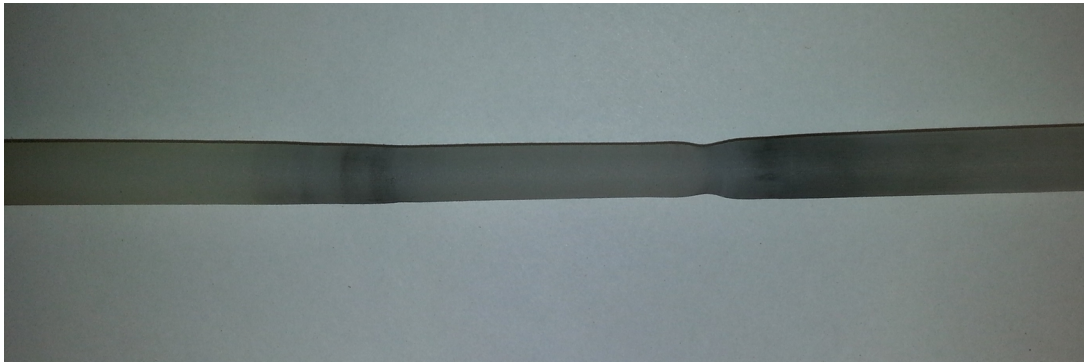
Pic 6-8: PA-6 rod fail
