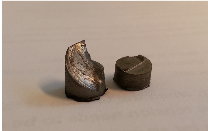
Pic 6-18: POM-C fracture surfaces. Sanded(l) and machined(r)
