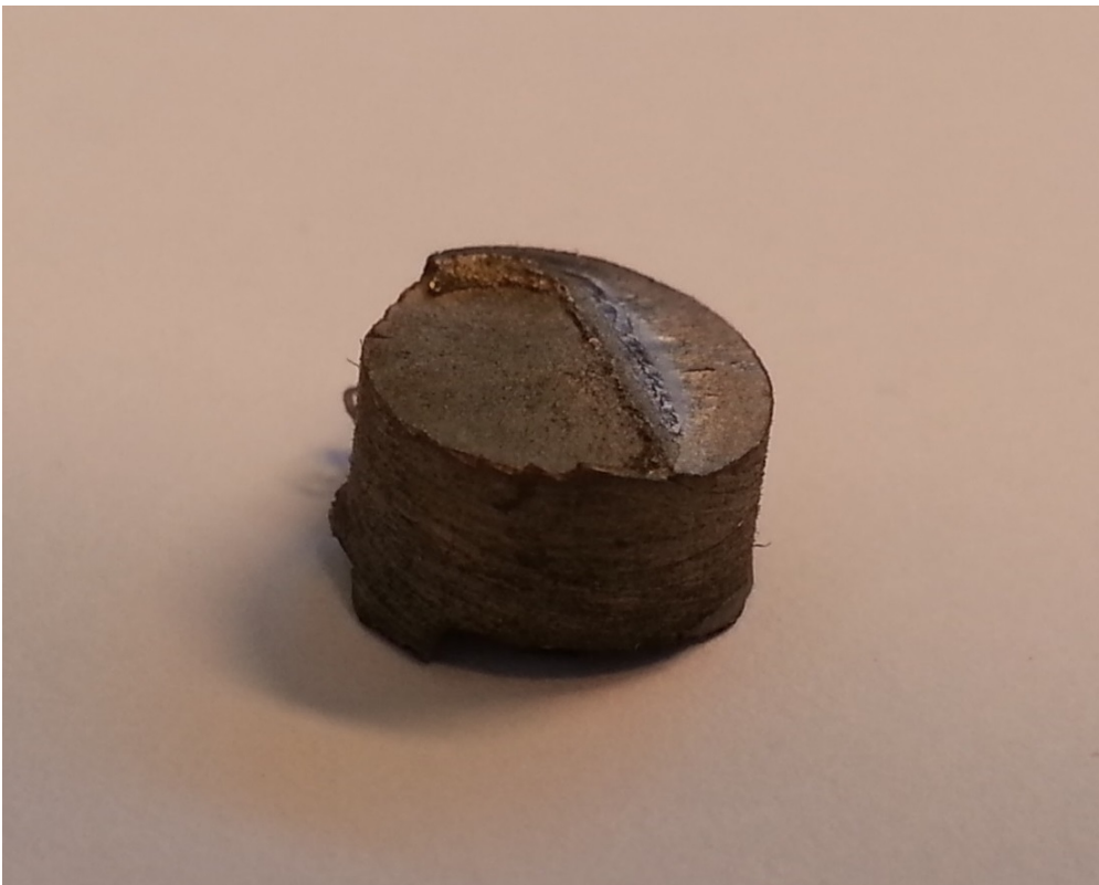
Pic 6-11: POM-C fracture surface
