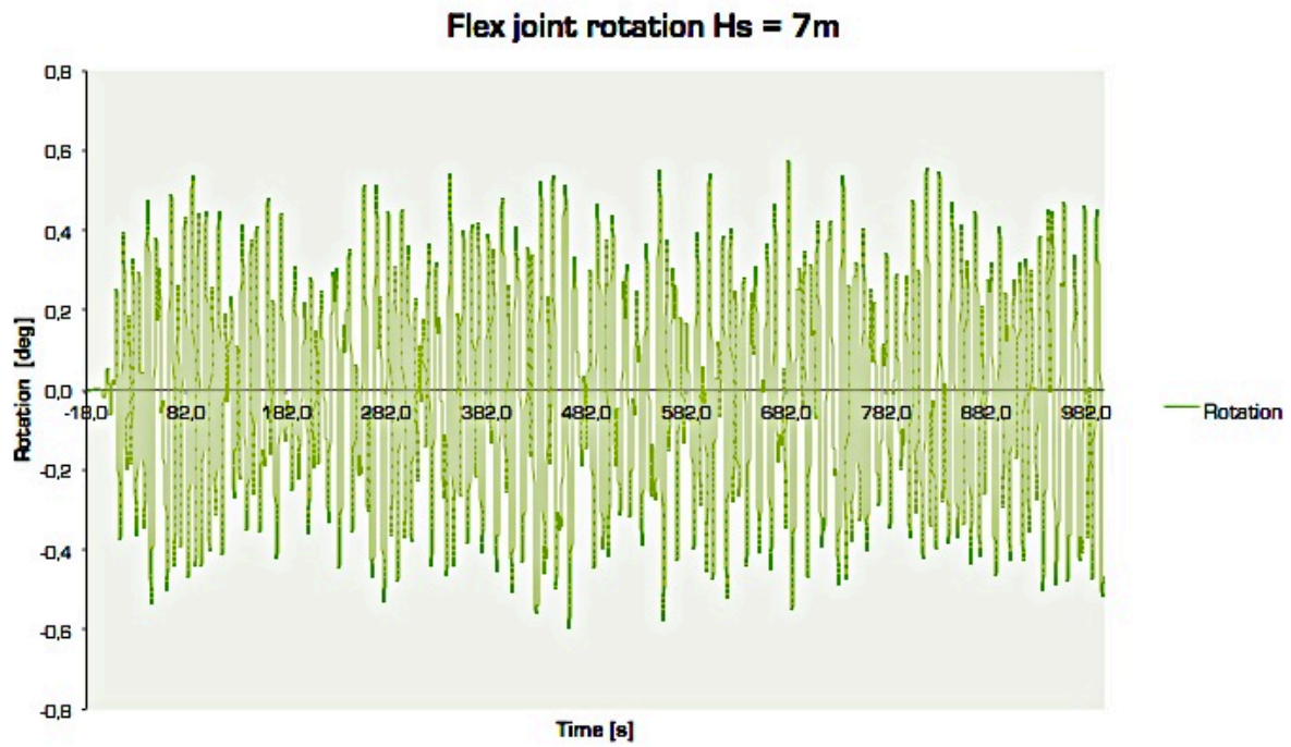
Figure C-2: Flex joint rotation as a function of simulation time (1000s), Hs=7m
