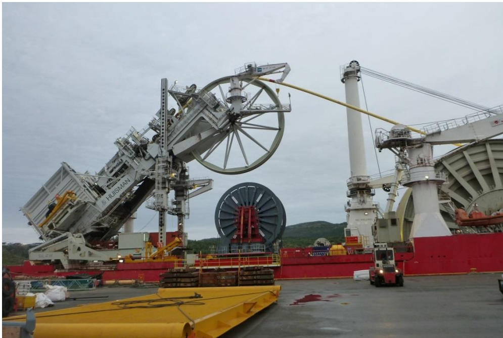
Figure 2-5: Pipeline over the Reel-lay vessel "Seaven Oceans" for residual curvature lay (Subsea 7, 2014)
