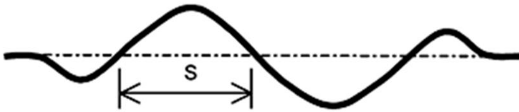
Figure 2-6: Typical Lateral Buckling Configuration (Einsfeld & Murray, 1984)
