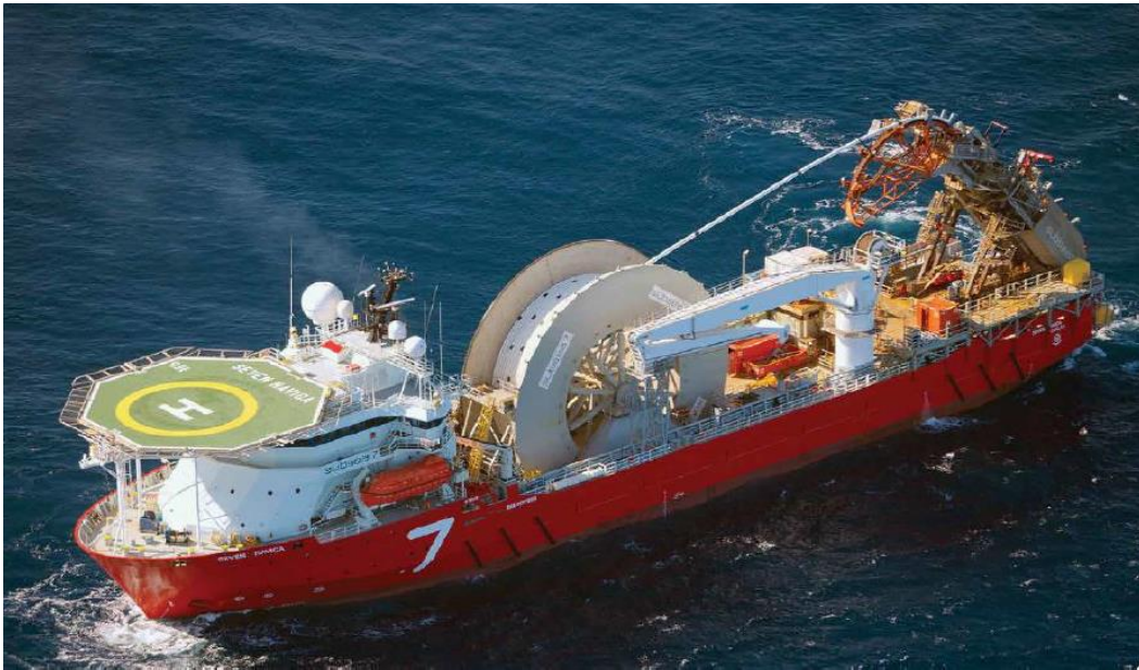
Figure 3-5: Reel-lay Vessel Subsea7's Seven Navica (Subsea7, 2012)
