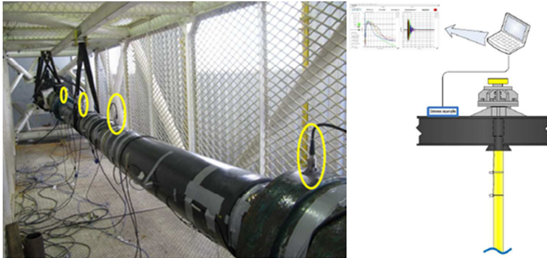
Figure 34 - Vibration monitoring laboratory test and field configuration [5].
