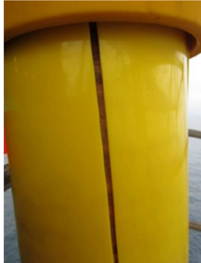
Figure 16 – Example of outer sheath cracking [1].
