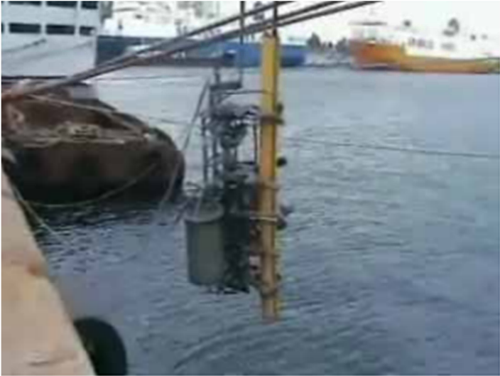
Figure 20 - Robot crawler with DR inspection tool [28].
