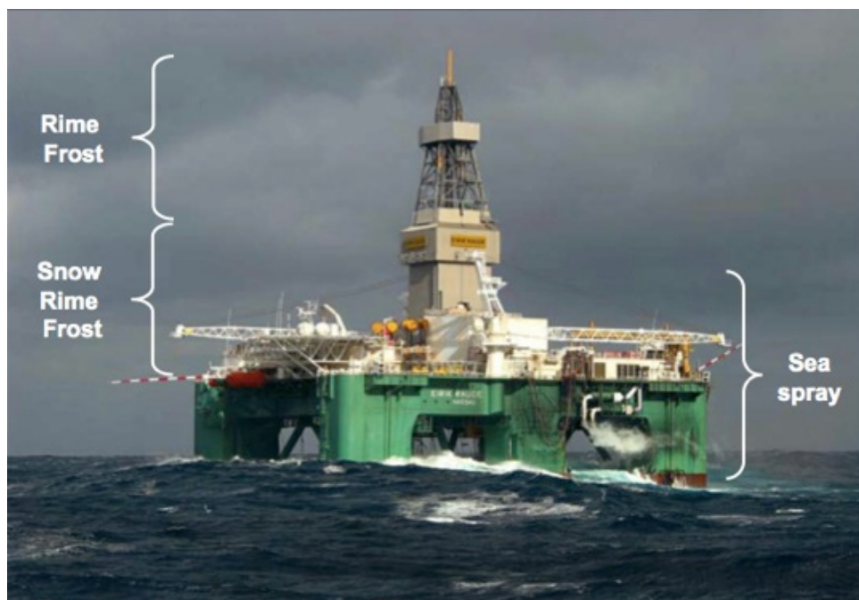
Figure 4.1-12 Areas of icing on a semi-submersible rig (Ryerson, 2011)
