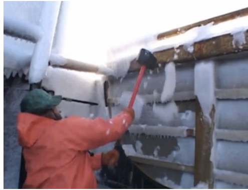
Figure 4.1-24 Manual de-icing on a crab fishing boat (Deadliest Catch. Man vs. Ice, 2006).
