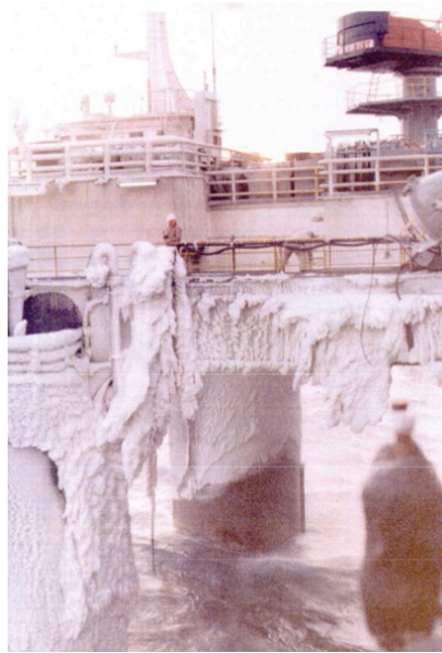
Figure 4.1-13 Sea spray icing the columns of a semisubmersible (Ryerson, 2013)
