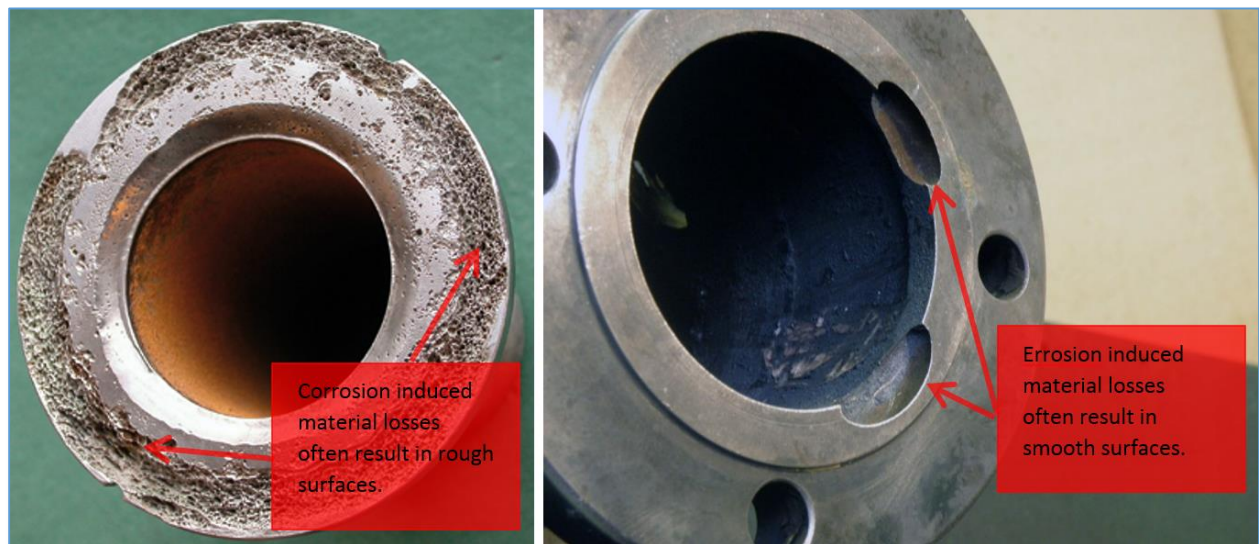
Figure B-2: Rough boundaries profiles compared to smooth boundary profiles generate more beam scatter affecting inspection results. The degree to which the beam scatter affects the final inspection results should be further studied.
