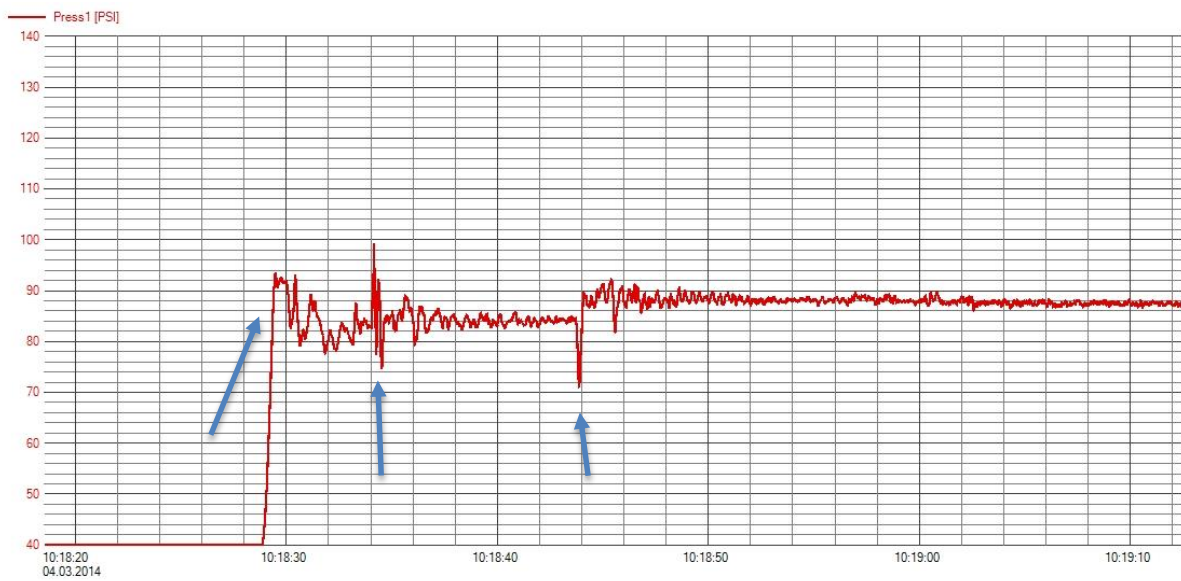
Figure 30 Run 2 04.03.2014 Samplings rate 1000 Hz Eztec TallyBook, signal from launch to arrival
