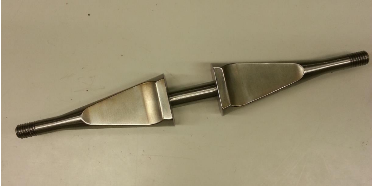
Figure 20: Anti-roll bar designed by M. Åsland.
