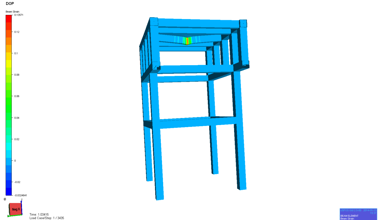
Figure 7.4 Strain in beam
