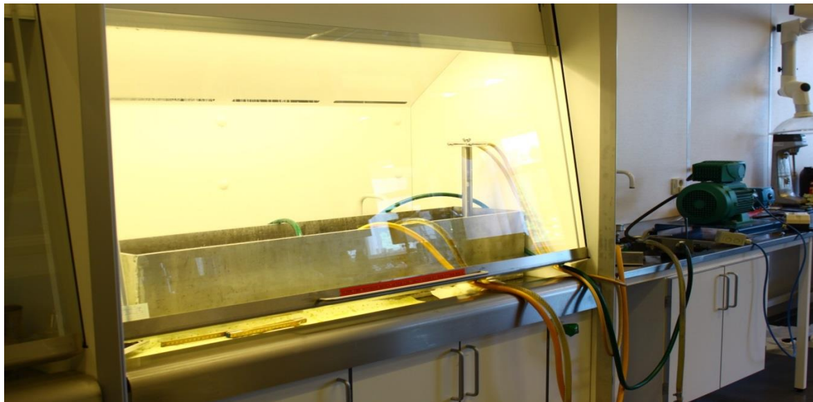
Figure 4.1a: Front view of experimental apparatus for fluid throw measurement.
