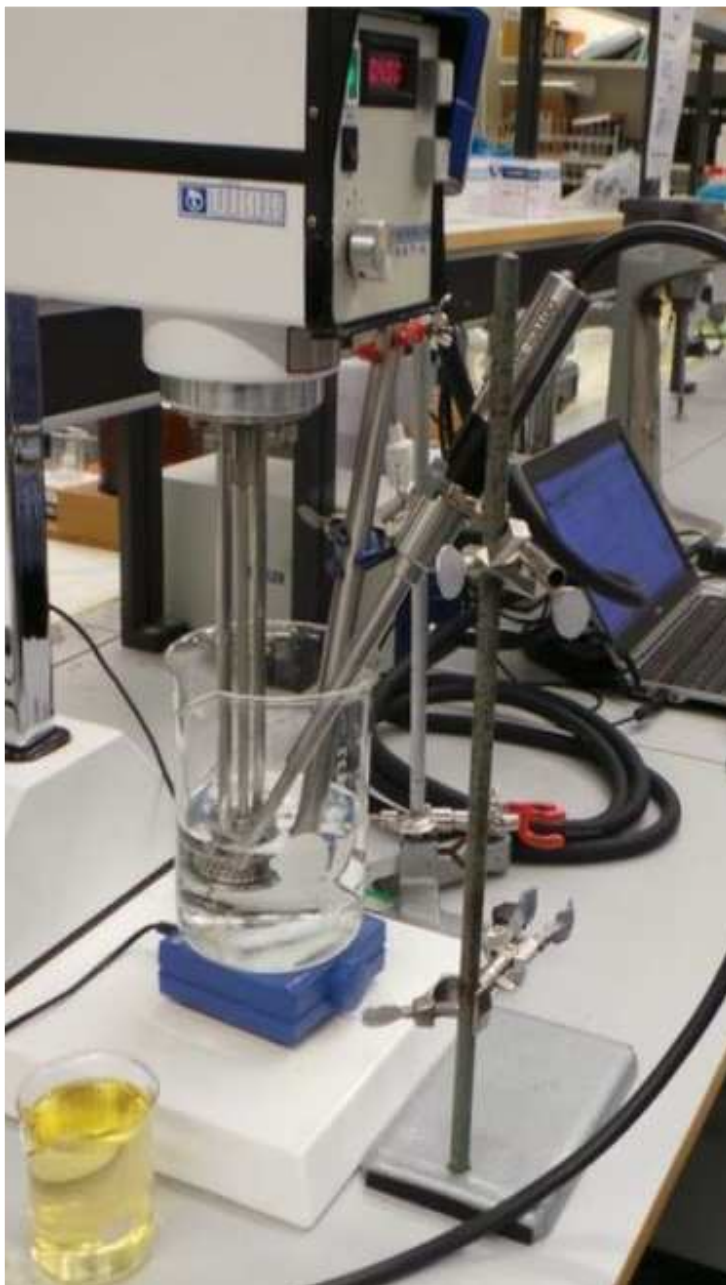
Fig. 24: FBRM and PVM experimental setup
