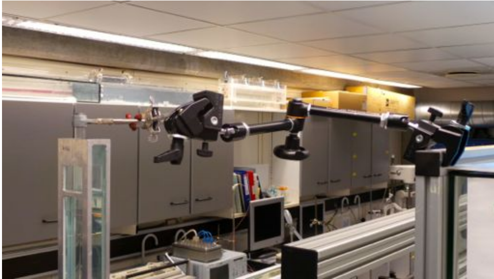
Figure C.2: Arms centralizing the inner pipe at the top
