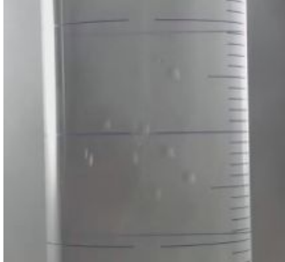
Figure 3.2: Dilute flow of 0.003 m glass beads in water
