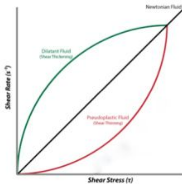
Figure 2.2: Comparison of Newtonian and non-Newtonian fluids [2]
