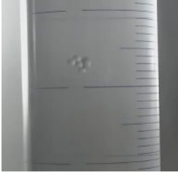
Figure 3.3: Dense flow of 0.003 m glass beads in PAC-4g/l
