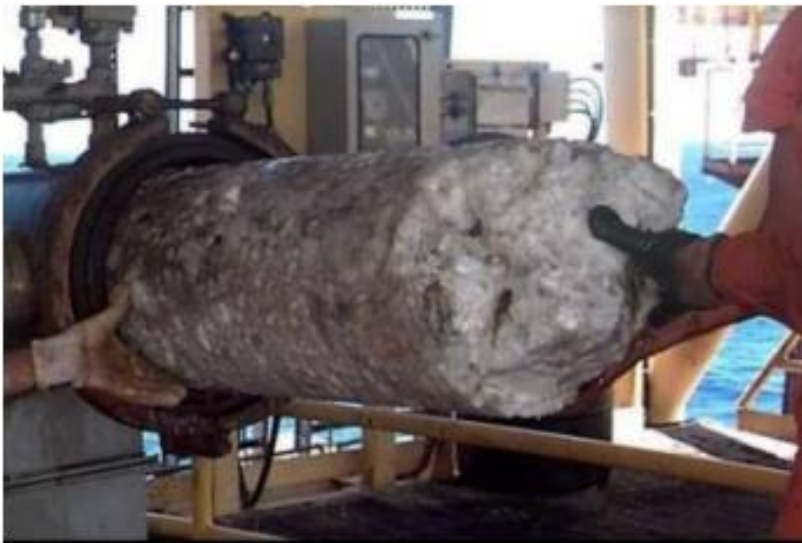
Figure 5.5 - Hydrate plug formed in subsea pipe offshore Brazil [13].
