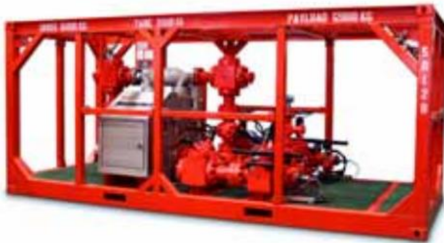
Figure 6.6 - A control system. Courtesy of Weatherford
