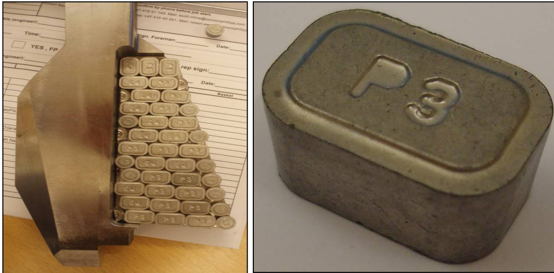
Figure 37: These two figures illustrate the P3 cutters (right side) and the mill (left side) [33].
