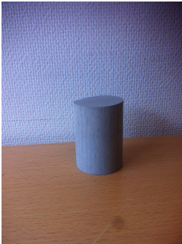
Figure 36: Sample of a rock based geopolymer from the University of Stavanger [23].
