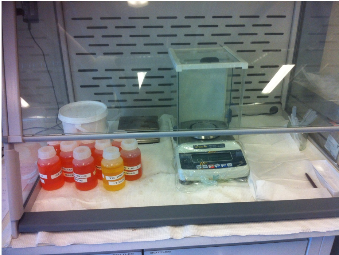
Figure 29: One of the chambers where the weight components and curing initiator are weighted [49].
