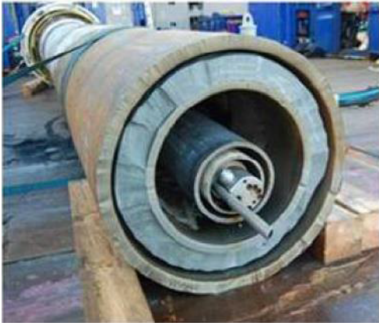
Figure 11: Retrieval of wellhead at Trolla [27].
