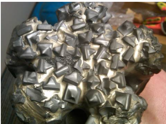
Figure 43: After 78 plugs, courtesy of Baker Hughes [33].
