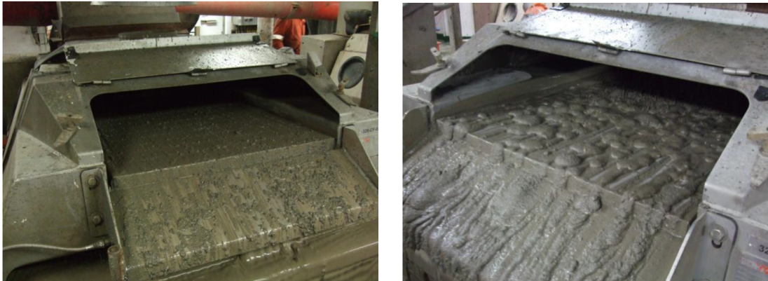
Figure 34: Normal well returns vs sand slurry returns [45].
