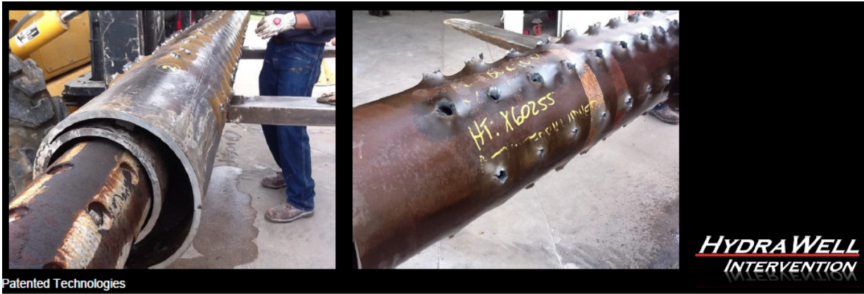
Figure 66: The picture above illustrates the “Burr” [20]. Burr is present on the outside of the casing as well as on the inside. The tools are therefore made with steel reinforced rubber cups so they can pass through the casing without being worn out (HydraWell 2014) [20].
