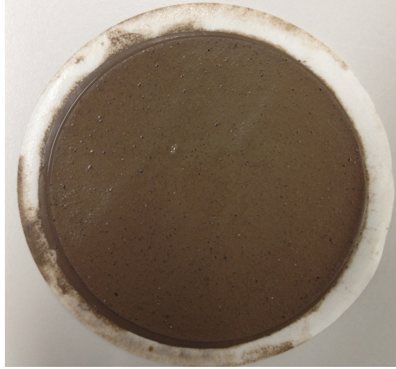
Figure 52. Filter cake of the C100 X1.4 B SW drilling fluid containing cuttings, xanthan and barite
