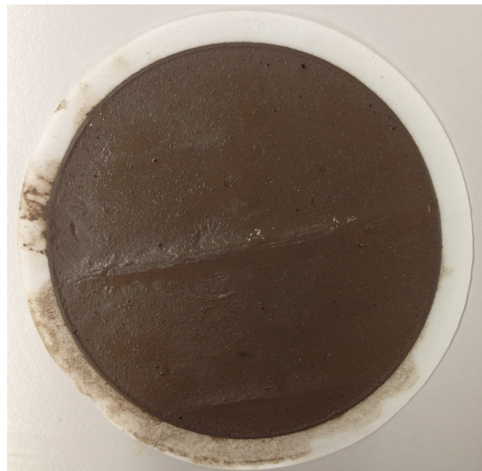
Figure 53. Filter cake of the C75 X1.4 CMC LV SW drilling fluid containing cuttings, xanthan and CMC Lo-Vis fluid loss agent
