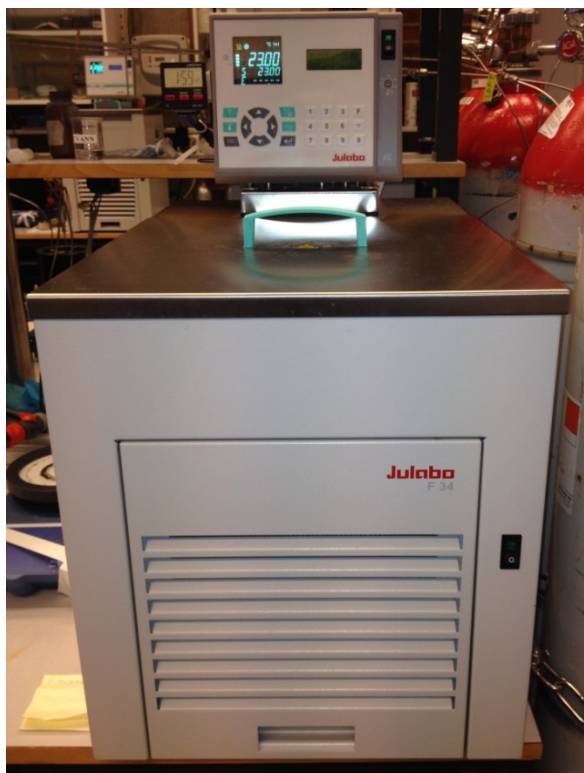
Figure 12 – Refrigerated - heating circulator Julabo F34-HL. The electronic timer is attached to the controlling block.
