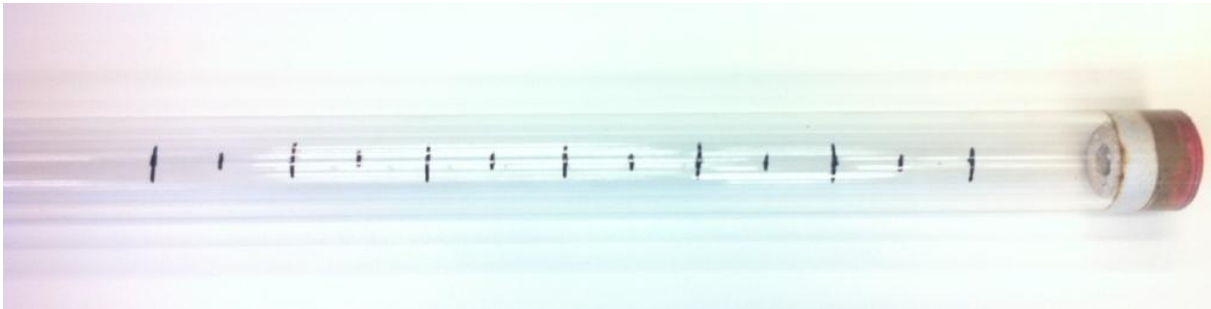
Picture C1: Displaying the acrylic tube with drawn measuring lines. Portrayed to the right is the polystyrene “donut” and the bottom plug. [01]
