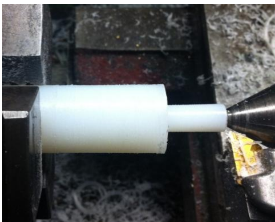
Picture C5: Showing the small tip being lathed and sanded down to correct size. [01]
