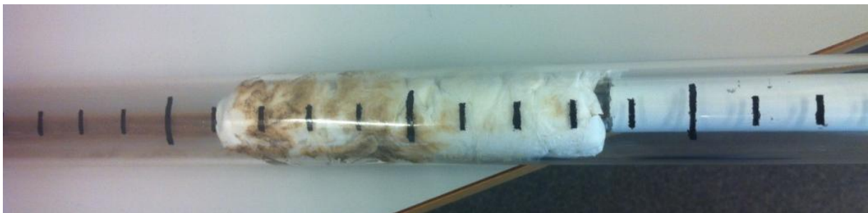
Picture C13: Displays the process of cleaning the long acrylic tube using paper towels as an improvised “Pig”. [01]
