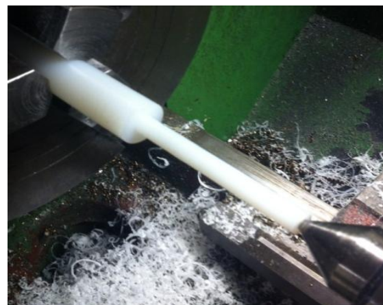
Picture C6: The rod positioned into the lathe after completing lathing the long tip. [01]
