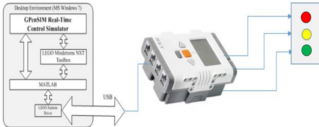
Fig. 30. Integration of Traffic signal system with GpenSIM
