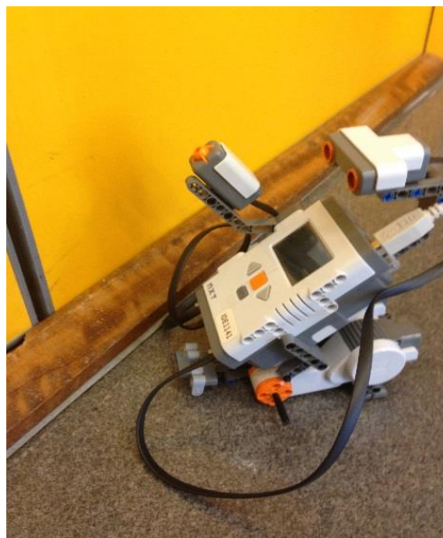
Fig. 21. A door alarm model using NXT and ultrasonic sensor
