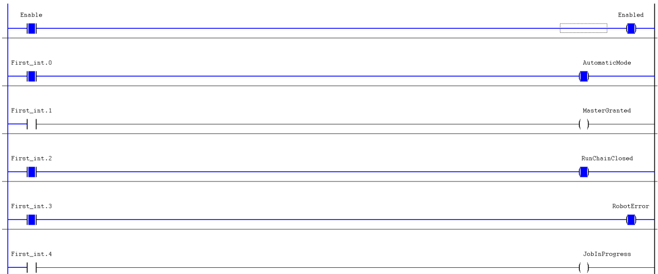
Figure 4.5: Extraction of boolean bits from a byte:
