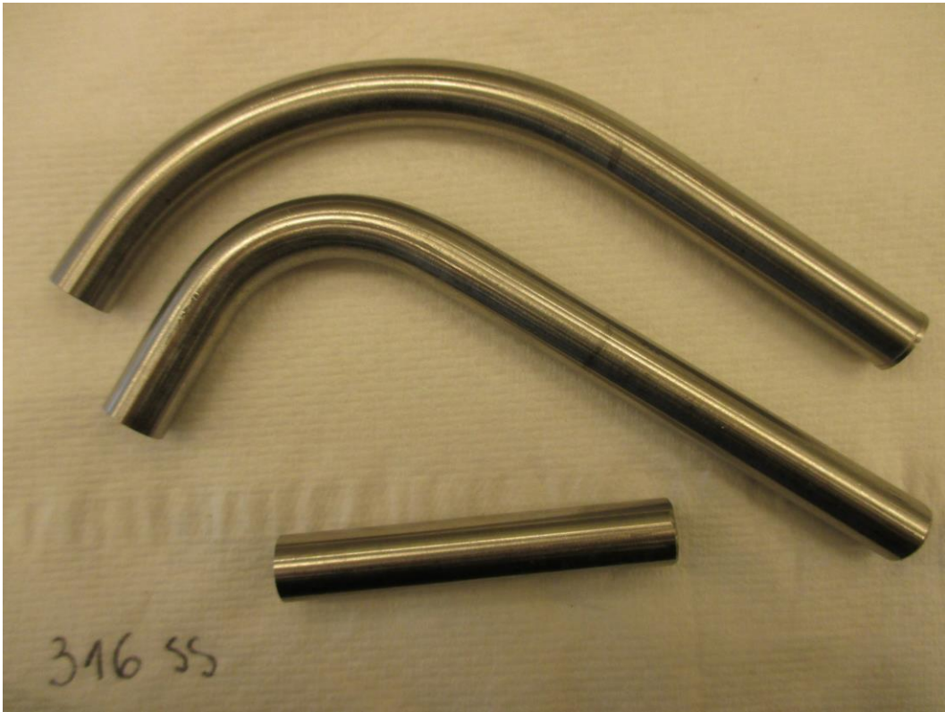
316SS specimens after G61 Test
