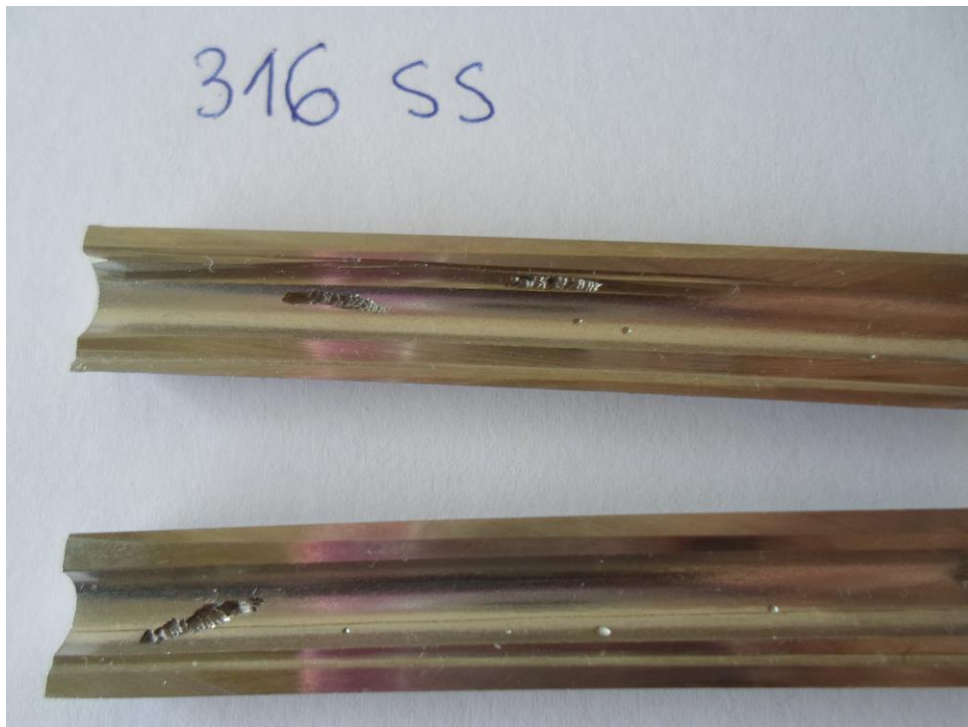
Inner surface of 316SS straight tubes after G48 test
