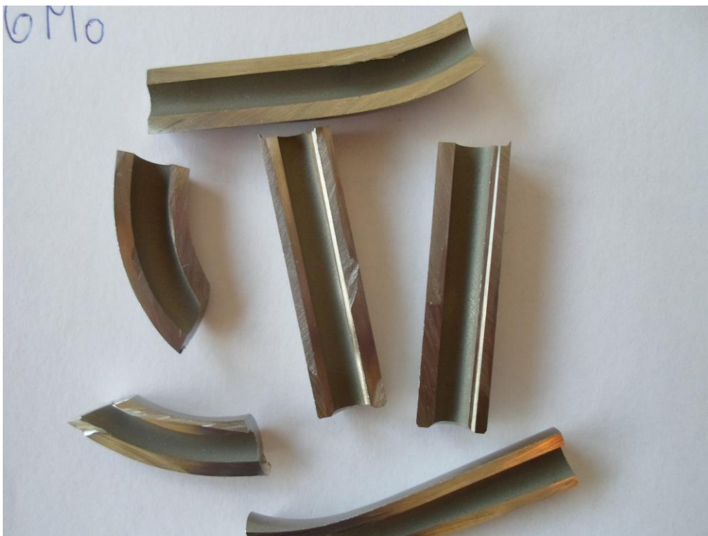
Inner surface of 6Mo bended and straight tubes after G48 test
