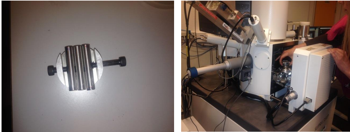
Figure 20: Samples ready for observation in SEM (Left) and placement in SEM (right)
