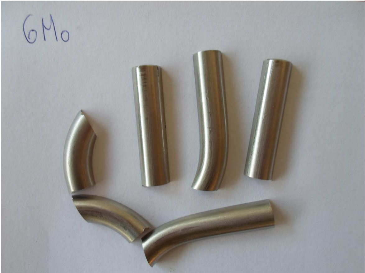
Outer surface of 6Mo bended and straight tubes after G48 test
