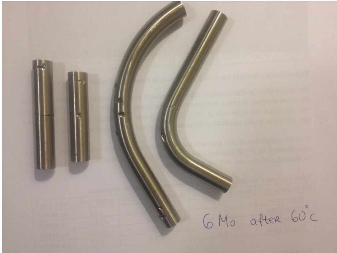
Figure 37: Specimens of 6Mo Stainless Steel after exposure to ferric chloride solution on 60° C
