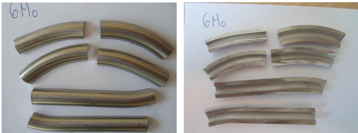
Figure 36: Outer (left) and Inner surface (right) of 6Mo specimens after G48 Test at 50°C
