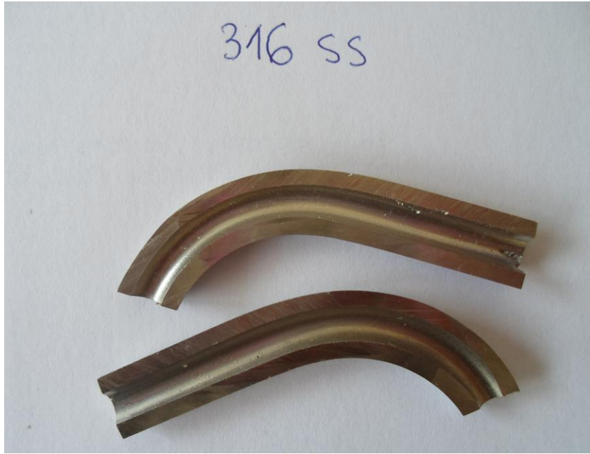
Inner surface of 316SS bended tubes after G48 test
